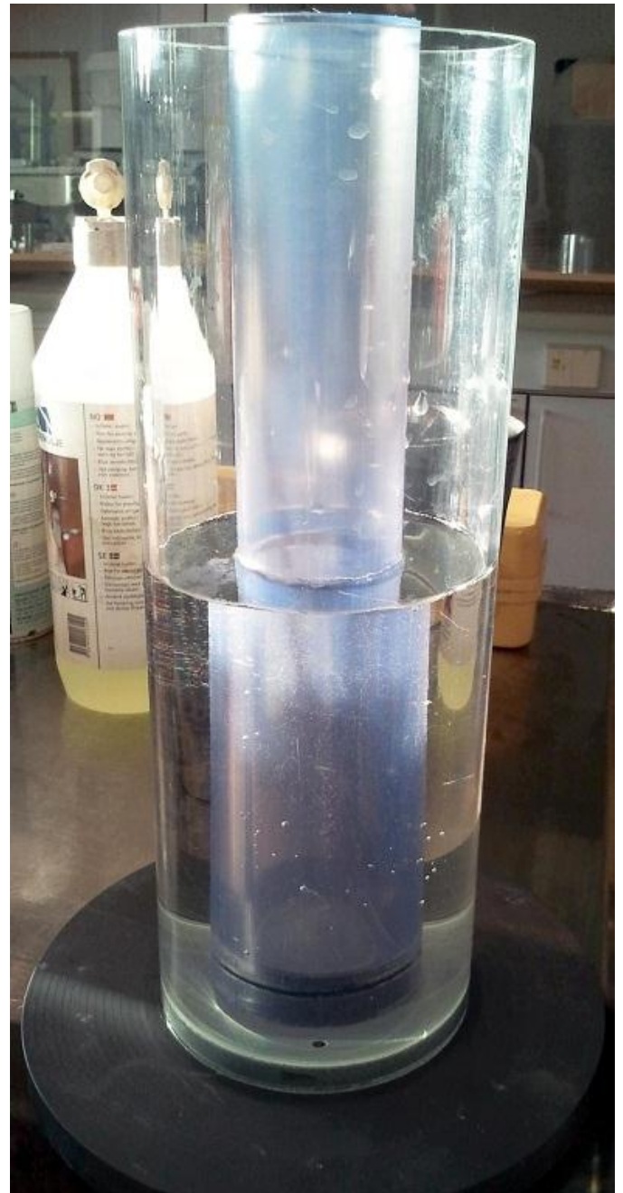
Figure 3.3: Old test pipe with a length of 30cm
