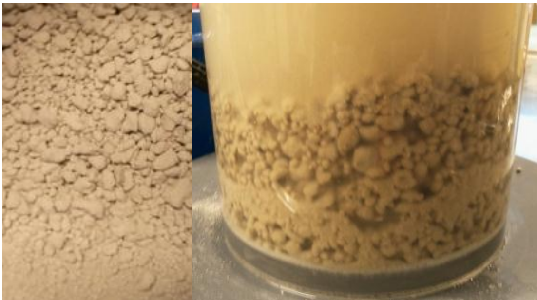
Figure 3.9: Left: Bentonite mixed with small amounts of water before adding to pipe, Right: Immediately after adding the mixed bentonite to a pipe filled with water
