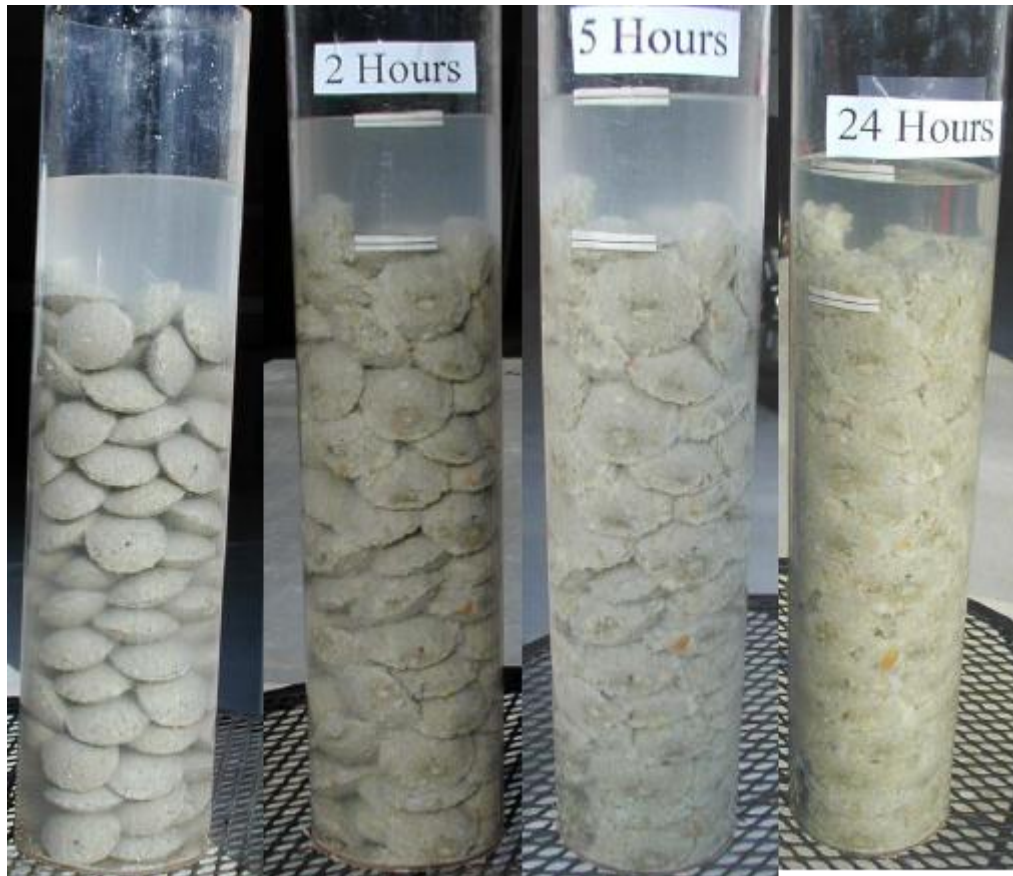
Figure 2.17: Hydration of compressed sodium bentonite nodules (Zonite) (Carl, 2004).
