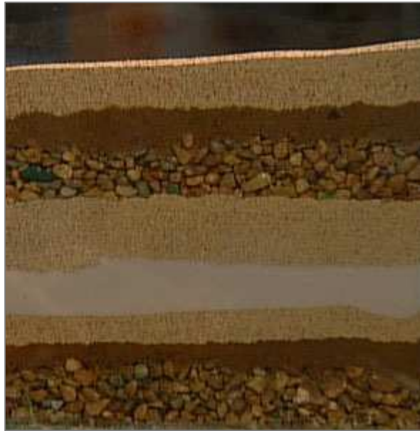
Figure 2-11: Model of the sedimentary process of deposition (Annenberg Foundation 2013). The alternation of layers is due to changes in the energy of the medium during the deposition.
