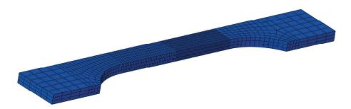
Figure 7.29: Mesh for simulations of rectangular PVC samples in uniaxial tension.
