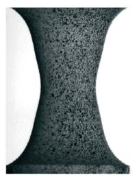
Figure 5.5: Representative image from tension test performed on a circular HDPE sample.
