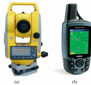
Fig. A 3 Leveling instruments: (a) Total station survey camera for height measurements, (b) GPSMap 60Cx used for horizontal location of the gravity points.
