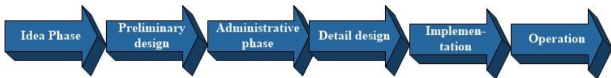
Figure 1 Phase stages in the scheme of the Polish road sector.
