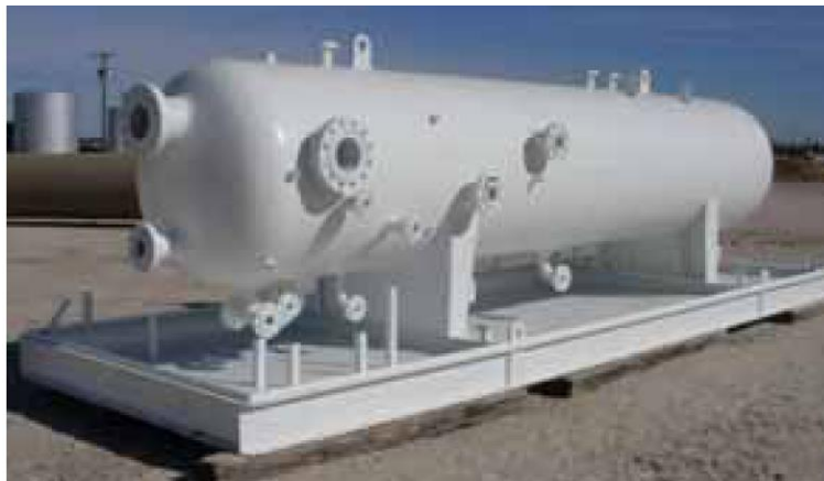
Figure 26-Horizontal gravity separator (Devold, 2013)
