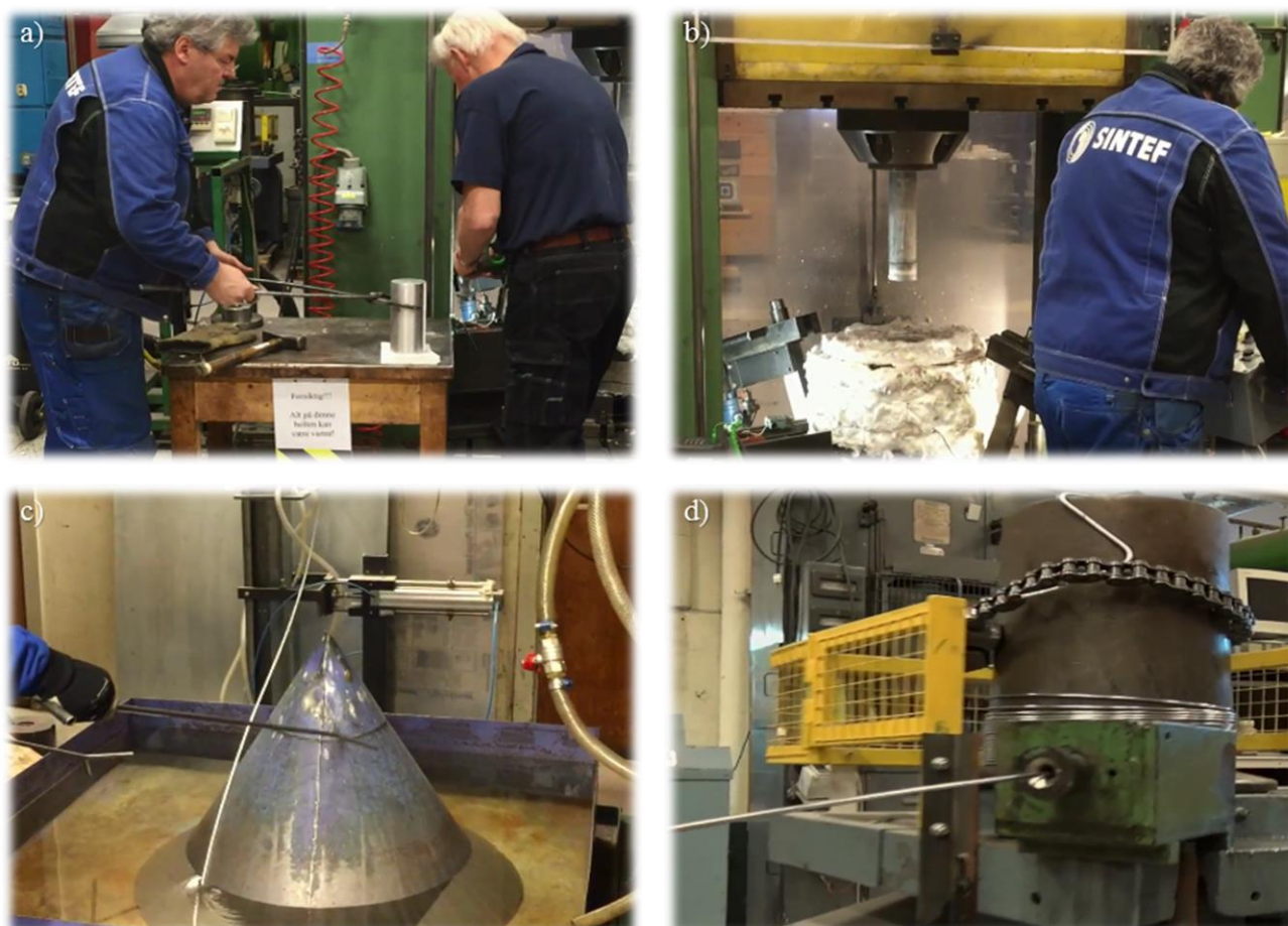
Figure 20 Illustration of the extrusion process: a) An ingot of re-melted traditional flush-mount anode with \text{\O}100 mm, b) The ingot is hot pressed through an orifice forming wire-die with \text{\O}5 mm. c) The hot pressed wire is produced and cooled and d) The wire is subsequently reduced to \text{\O}2 mm for thermal spraying.
