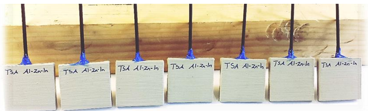
Figure 23 DSA specimens connected to a 3 mm insulated threaded rod, ready for exposure (the painted sides of the specimens are shown). Notice that the specimens are called TSA Al-Zn-In. This was before it was decided to name the new coating system for DSA.
