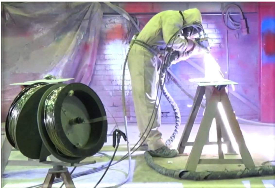
Figure 21 Coatings applied using electric arc spray.
