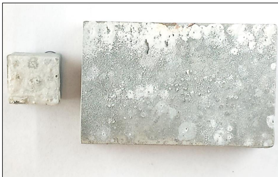
Figure D. 4 Galvanic Couplings before and after 30 days of exposure to natural seawater at 40 \pm 5^\circ\text{C}
