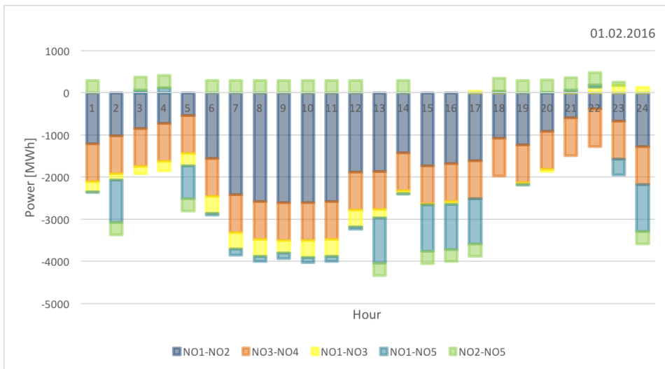
Figure A.2: Case 2: Power flow between areas, congestion line 4 to 785 MW, with battery in node 1, 01.02.2016.
