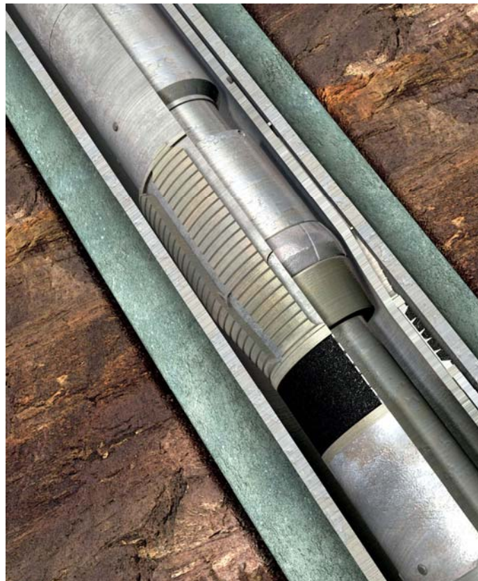
Figure 40: TORXS expandable liner hanger during expansion 10
