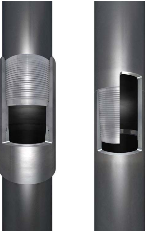
Figure 15: Coupling connection (left) and integral connection (right) 7
