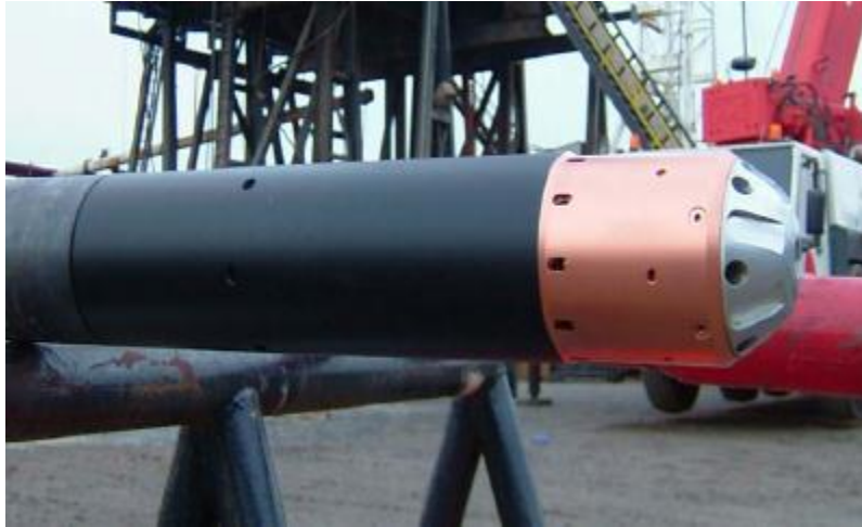
Figure 2.12: Flow diversion shoe (Howelett et al. 2006).
