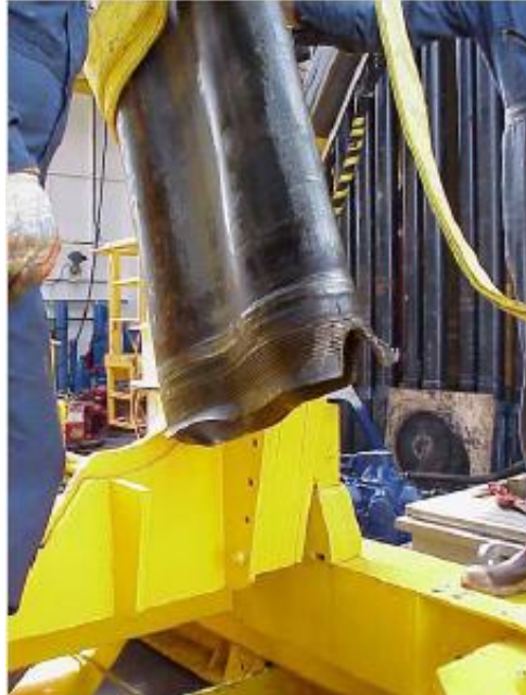
Figure 3.4:Collapsed casing string (George E. King Engineering, 2009).
