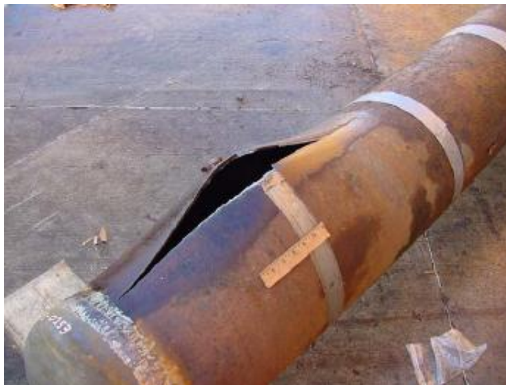
Figure 3.1: Burst casing (George E. King Engineering, 2009).
