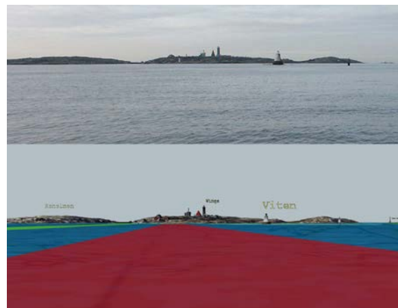
Figure 5: A photograph from a boat approaching Vinga lighthouse. The camera is placed 2 meters above the water. Bottom, the same view in the egocentric 3D map.
