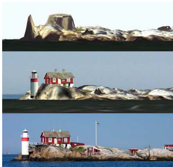
Figure 6: Top, the raw interpolated LIDAR terrain model. Middle, the manually modelled beacon and building added in 3ds Max. Bottom, a photograph from the actual site.
