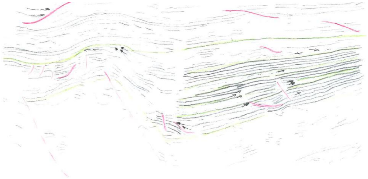
Figure 5.7 Line NH8802-32 with main boundary surfaces in green and faults in red. Arrows indicate terminations of reflectors.
