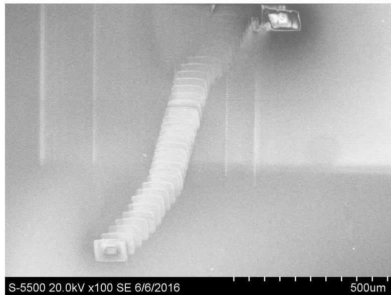
Figure 6.14: A S(T)EM photo where charge effects can be seen.
