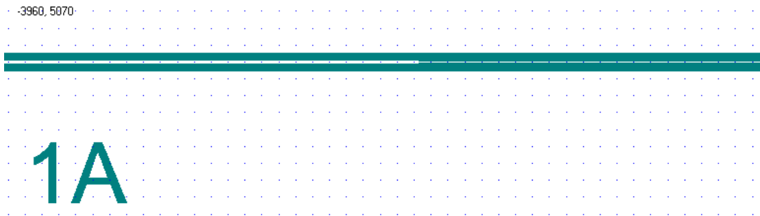
Figure 4.6: A clipping of a taper at the beginning of a waveguide. The white part is the waveguide and the green part on the sides are the 8 \mu\text{m} wide exposed area.
