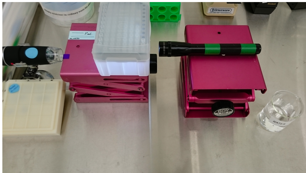
Figure 3.4.4: Contact angle measurement setup with the HOT USB microscope to the left, adjustable sample stage with a 10 \times 10 \text{ mm}^2 sample, and a primitive halogen light source to the right. A plastic box was used as a light diffuser.
