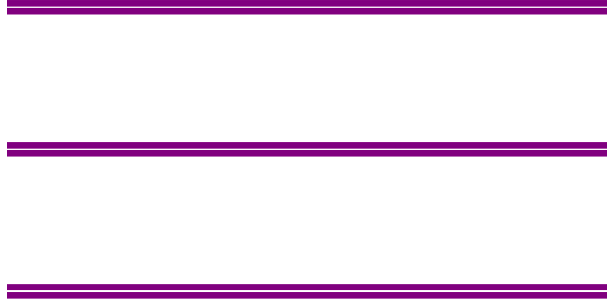
Figure 3.2.3: Magnified image illustrating an inverted mask in CleWin4. The purple areas are to be exposed and further etched, resulting in light-confining ribs (white lines).
