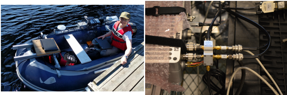
Figure 6.12: To the left, both system are mounted on same rigid frame. To the right a DC block to ensure only one system powers the antennas.
