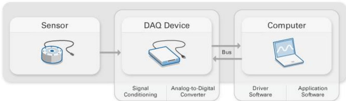
Figure 3-9 Parts of a DAQ system. (Instruments N.A)
