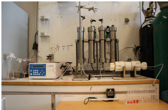
Figure B.3: Flooding apparatus - Picture of set up of flooding apparatus. Pump connected to three out of four cylinders containing brine, oil and Aerosil300 nanofluid
