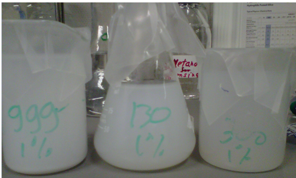
Figure B.1: Stabilization analysis of nanofluids - Stabilization analysis of three different nanoparticles in brine prepared with 1wt% solution. From the left Elkem 999, Aerosil130 and Aerosil300.
