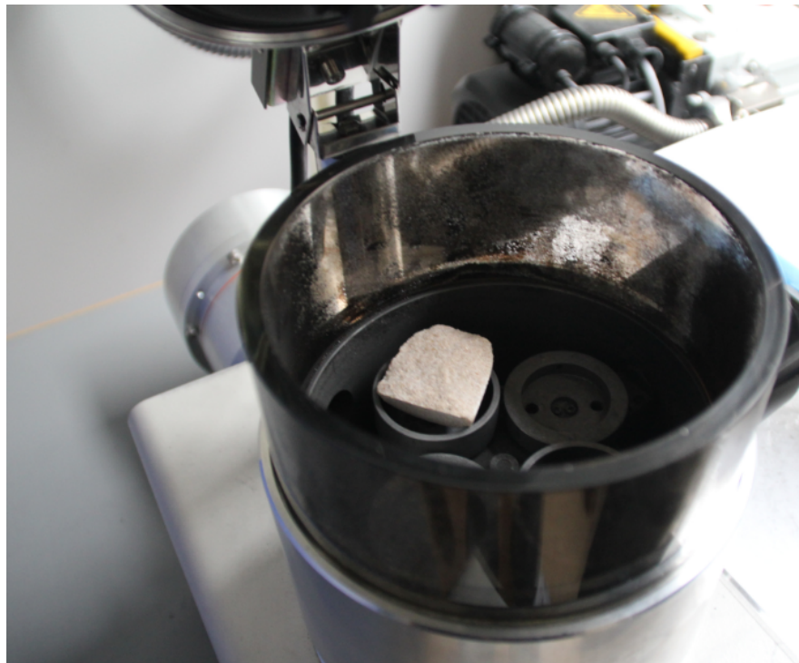
Figure B.8: Carbon-coater - Core sample placed inside carbon-coater
