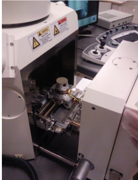
Figure B.6: Core inside SEM - A core sample placed on solid surface inside SEM for analyzing
