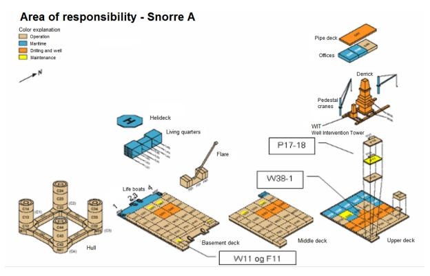
Figure 4.7: The figure shows different modules on the rig, highlighting the modules were gas was detected (Brattbakk et al., 2005).
