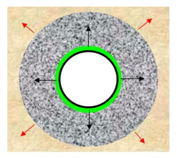
Figure 2.7: The figure shows the effects on the cement when the formation has a lower Young's modulus than the cement (Bouras et al., 2008). Here a micro annulus is created as shown in green due to cement expanding outwards.
