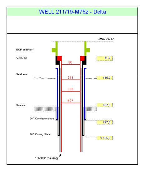
Figure 5.4: The figure illustrates in which area of the well the jarring took place when the 20" casing failed (between 80 and 211 ft). All depths are shown in feet (RevusEnergy, 2008).
