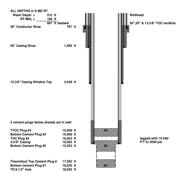
Figure 5.2: The figure shows the status of the M-75 well prior to the slot recovery startup (CNR, 2008).
