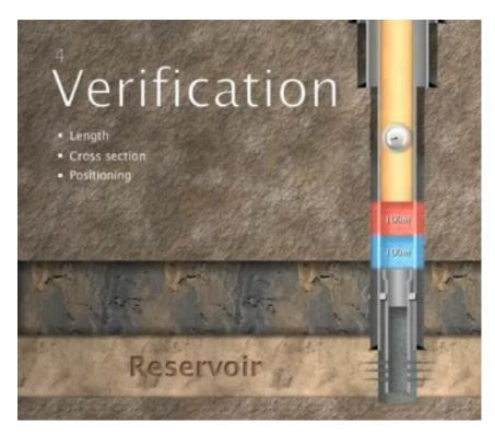
Figure 2.15: The figure illustrates a pressure test on the barriers. This is done to verify the integrity of the barriers (Statoil, 2011b).
