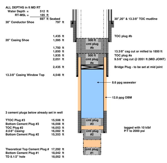
Figure 5.3: The figure shows the M-75z abandonment design after the slot recovery of the M-75 (CNR, 2008).
