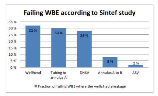
Figure 2.5: The chart illustrates in which WBE the integrity issues occurred in the wells which experienced leakage (Randhol & Carlsen, 2007).
