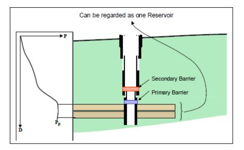
Figure 2.16: The figure shows two separate reservoirs where there pressure in the deepest reservoir is either equal or less than the pressure in the shallower reservoir. They can therefore be regarded as one reservoir in an abandonment perspective (NORSOK, 2011).
