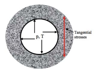
Figure 2.6: The figure shows stresses on the cement when the casing is expanding (Goodwin & Crook, 1992).
