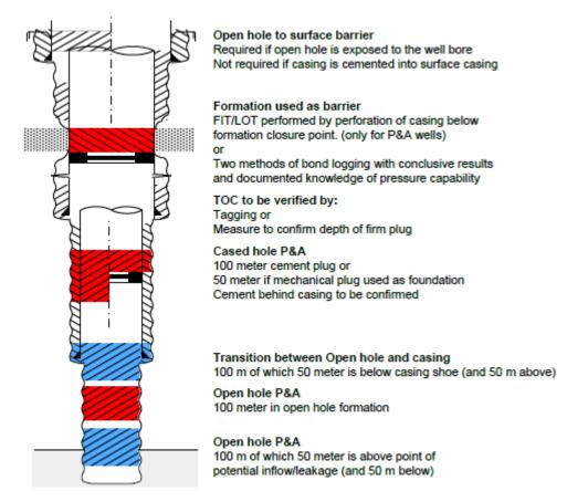
Figure 2.10: The figure shows cement plug criteria as per NORSOK D-010 (WellBarrier, 2012b).
