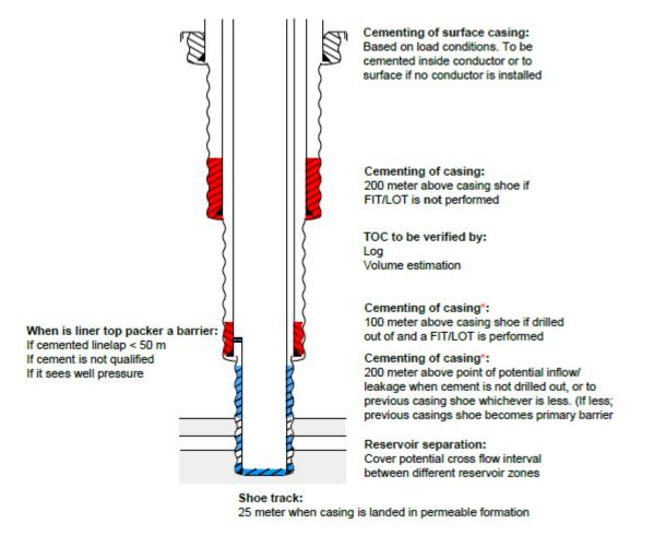
Figure 2.13: The figure shows different casing cement requirements as per NORSOK D-010 (WellBarrier, 2012b).
