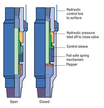
Figure 4.4: The figure shows in a simple way the principle of a down hole safety value in an open and closed position.
