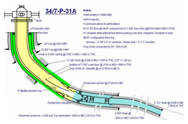
Figure 4.5: The figure shows status before the incident took place. The most notable things to observe is the punched hole in the tail pipe and the hole in 95/8" csg at 1561 m MD (Brattbakk et al., 2005).
