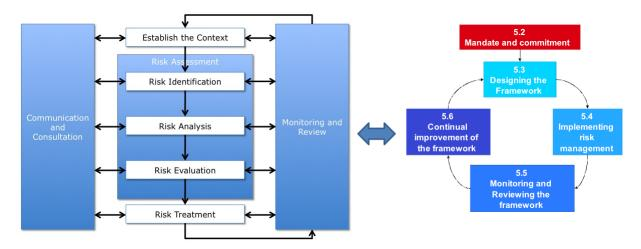
Figure 3.3: The figure illustrates the connection between the different processes in risk management on the left and the framework on the right. The figure is based on models found in (ISO, 2009).
