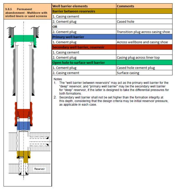
Figure A.5: Barrier requirements for cased hole scenario on the right and the use of a transistion plug on the left (NORSOK, 2011).
