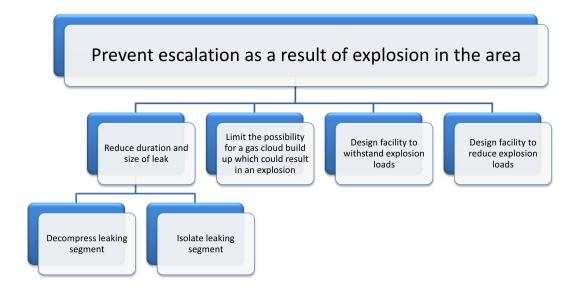
Figure 3.1: The figure shows a hierarchy of barrier functions, and how certain barrier functions are dependent of the implementation of other barrier functions.
