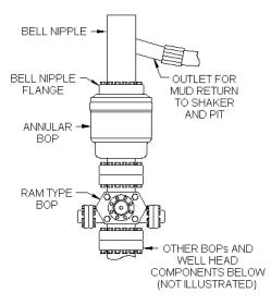
Figure 4.8: The figure shows a simple schematic of where the bell nipple is located (Co USA, 2011).
