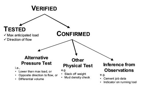
Figure 3.5: The figure shows different ways to either verify or confirm in-situ barriers (BSEE, 2011).
