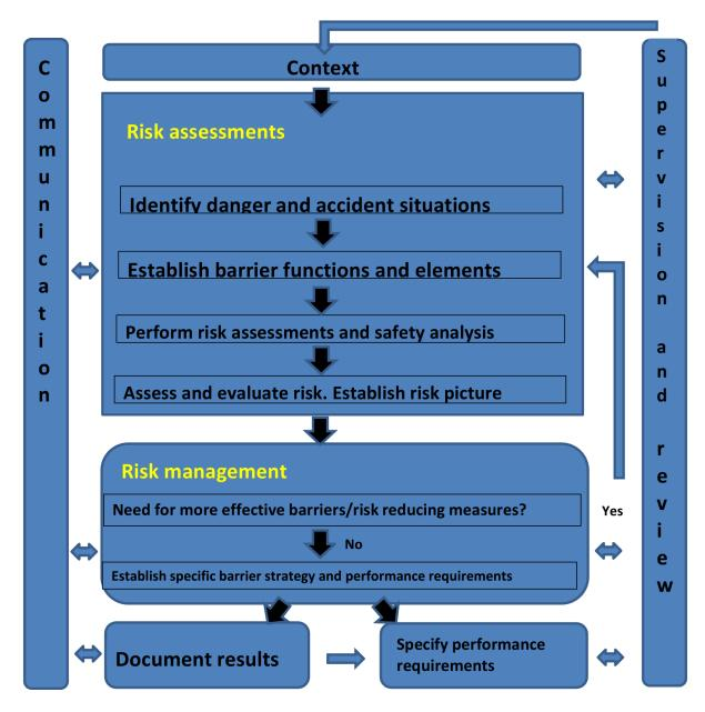
Figure 3.4: The figure shows a barrier control process with the planning phase in focus. The model is based on models found in (PSA, 2012a) and (ISO, 2009).
