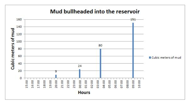
Figure 4.11: This graph shows the amount of mud bullheaded into the formation. These numbers are inserted into figure 4.10 to give a more precise view of how the pressure behaved when bullheading mud.
