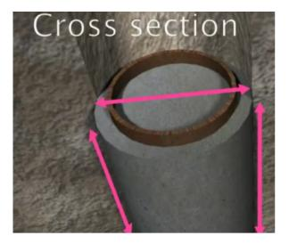
Figure 2.12: The figure shows what it looks like when the well is correctly sealed both across the cross section and vertically and horizontally (Statoil, 2011b).
