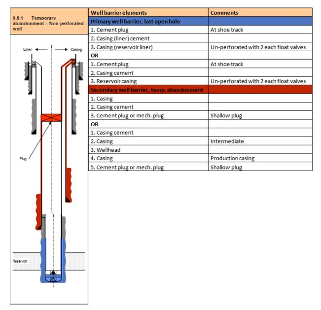
Figure A.1: Barrier requirements for liners on the left, and barriers for casings on the right (NORSOK, 2011).
