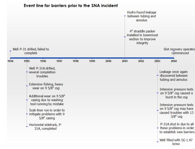
Figure 4.14: The figure shows a time line of how the barriers developed prior to the slot recovery operation start-up in 2004.
