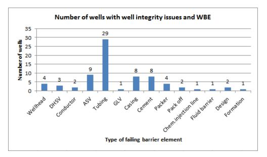
Figure 2.3: The chart illustrates in which WBE the wells with integrity issues experiences problems. Tubing related issues is by far the most distinct problem.
