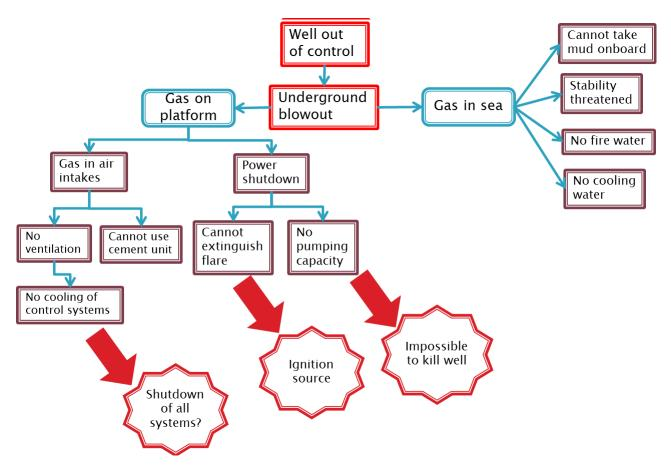
Figure 4.13: A slightly more complex schematic of how the problems developed on the rig itself, and how limited measures for the crew were.
