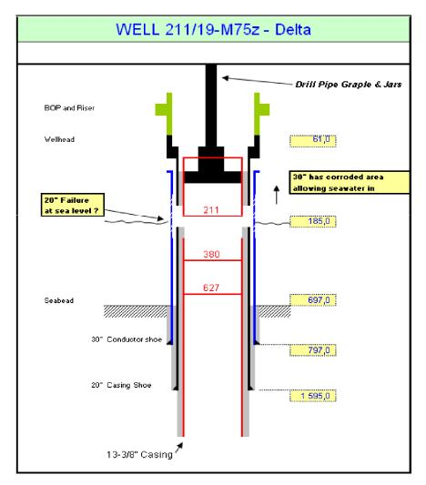
Figure 5.5: The figure illustrates where the 20" casing failed (around sea level). All depths are shown in feet (RevusEnergy, 2008).
