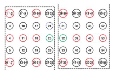
Figure 1.1: The figure shows a 40-slot surface layout, which with combined conductor sharing allows 56 wells to be drilled. Wells include cutting/re-injection candidate wells in green, cellar deck wells shown in red and mez-zanine decks wells shown in black (Fu et al., 2009).
