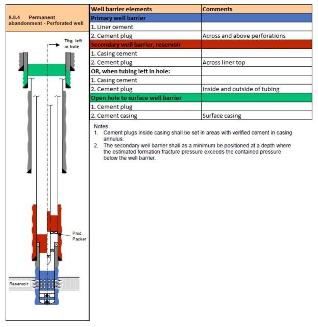
Figure A.4: Barrier requirements for liners on the left, and barriers when the tubing is left in the hole on the right (NORSOK, 2011).
