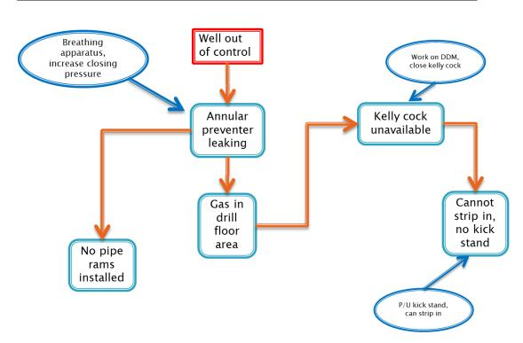
Figure 4.12: The schematic shows in a simple way the causes and consequences to the problems on the drill floor.
