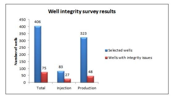
Figure 2.1: The chart illustrates how many of the selected wells which experienced well integrity problems.
