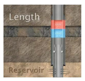
Figure 2.11: The figure shows a cement plug which has acceptable contact to a fundament, and also one which does not meet the acceptance criteria (Statoil, 2011b).
