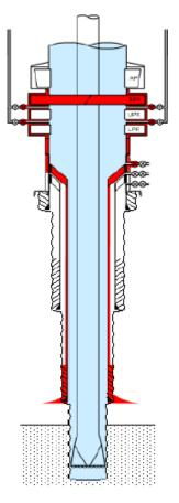
Figure 2.9: In a well drilling situations we see that the fluid column is acting as a primary barrier (blue color), and the secondary barrier (red color) represents the *envelope* consisting of casing, casing hanger, wellhead and BOP with the closed blind/shear rams (WellBarrier, 2012a).
