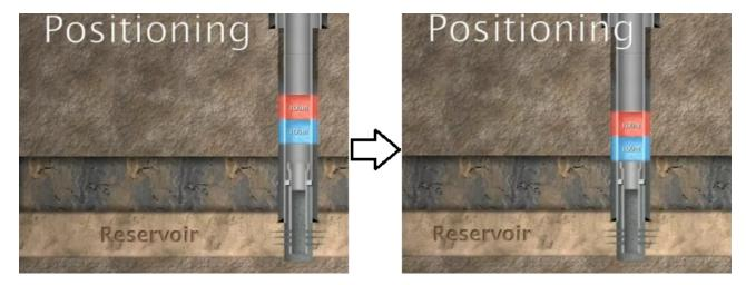
Figure 2.14: The figure shows how to correctly position the barriers. In the case on the left the barrier is placed too shallow, and should be moved deeper as illustrated on the right (Statoil, 2011b).
