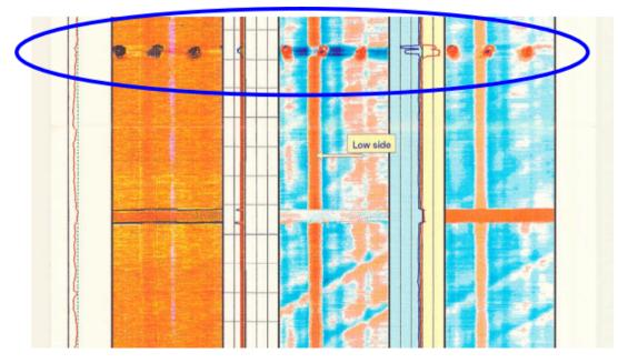
Figure 4.2: The figure shows the three holes created by the high-pressure washing tool. The image is created from a USIT/CBL log (Brattbakk et al., 2005).
