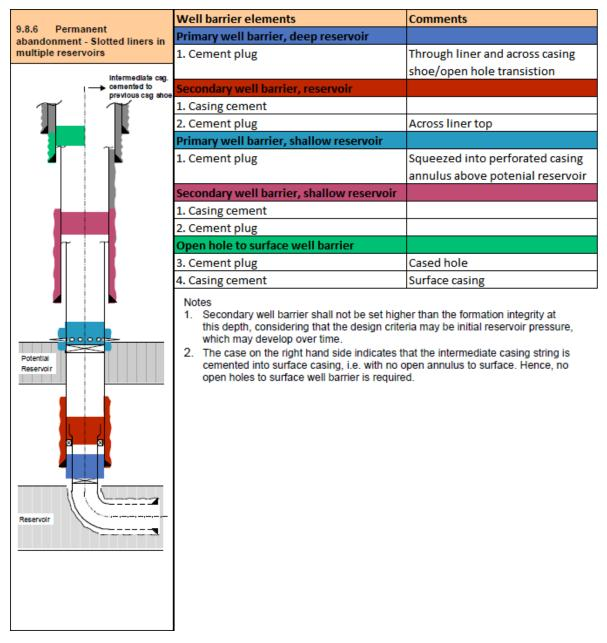
Figure A.6: Barrier requirements for intermediate casing cemented to the previous casing shoe on the right (NORSOK, 2011).
