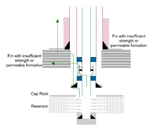
Figure 2.8: The figure shows a well barrier envelope which would qualify for the "red" category (OLF, 2010).
