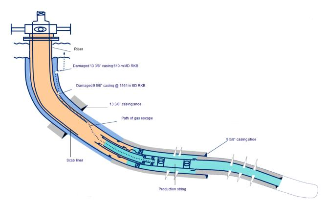
Figure 4.6: The figure shows how the gas escapes the wellbore through damaged parts of the casing (Petersen et al., 2006).
