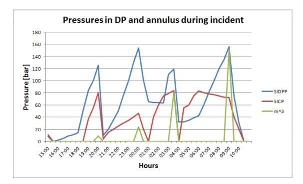
Figure 4.10: The graph shows how the SIDPP and SICP behaved during the incident. The green curve shows when mud was bullheaded into the formation.
