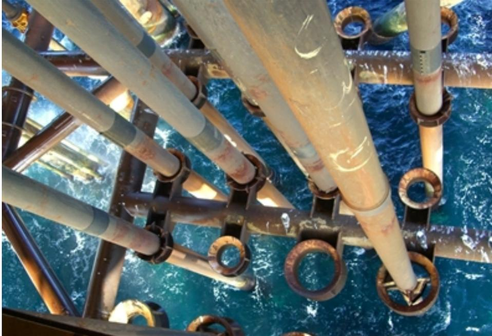
Figure 1.2: The figure shows how a slot layout on a platform looks like. Note that there are several free slots on this platform (Claxton, 2012).
