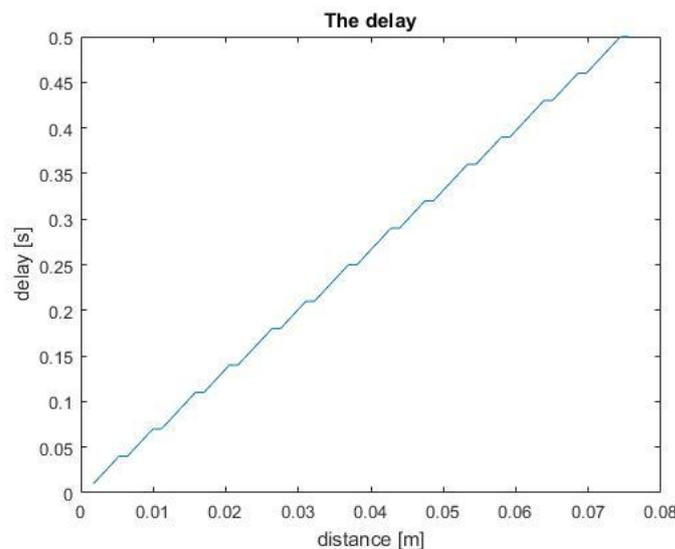
Figure 18: The delay of the concentration in the deterministic SISO communication system
