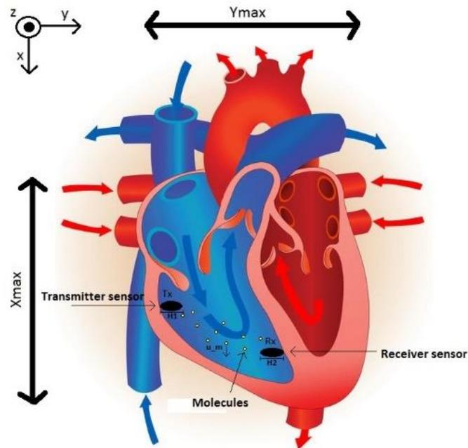
Figure 6: A model of the heart with the pacemaker system implemented [49]
