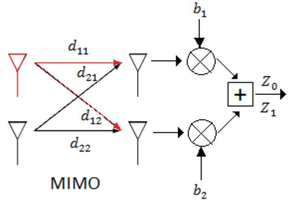
Figure 14: The MIMO system part 2 where transmitter 2 is considered
