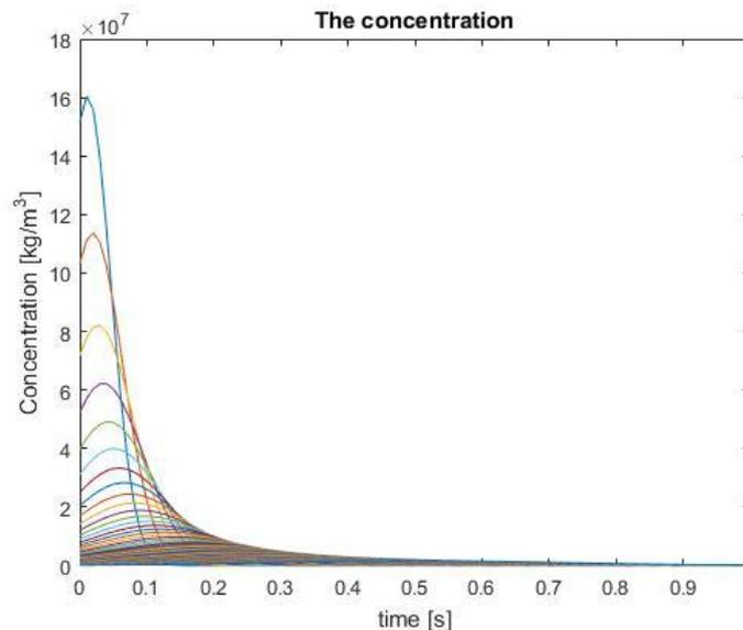
Figure 16: The concentration of the molecules in the deterministic SISO communication system dependent on the distance travelled by the molecules in the  $x$ -direction in meters and the time in seconds, where each curve represents different distances
