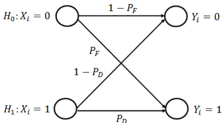
Figure 9: Binary hypothesis testing channel
