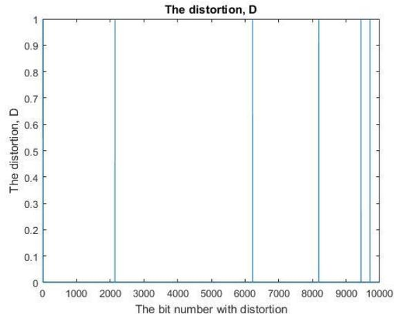
Figure 29: The distortion,  $D$  s with the stochastic SISO communication system and signaling interval  $T_s = 200$  s
