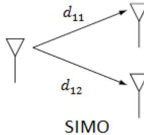
Figure 10: SIMO communication system with distances  $d_{11}$  and  $d_{12}$  between the transmit and receive antennas
