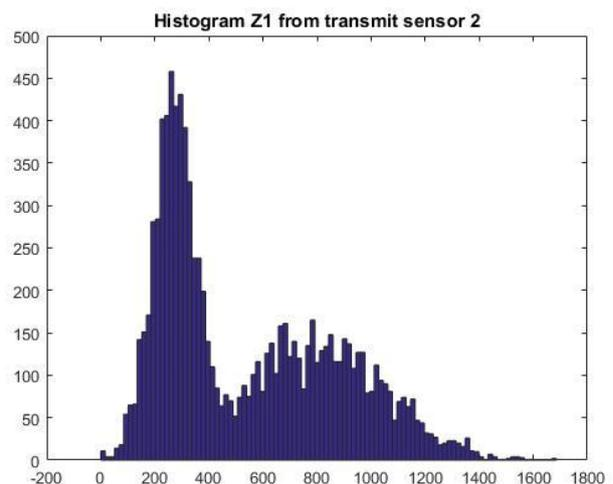
Figure 55: The distribution of  $Z_1$  from transmit sensor 2 with MIMO communication and the signaling interval,  $T_s = 300$  s
