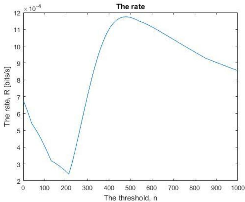
Figure 39: The rate, R with the stochastic SIMO communication system when  $T_s = 200$  s
