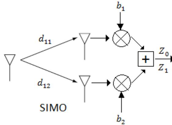
Figure 11: The SIMO communication system with use of the diversity technique, MRC
