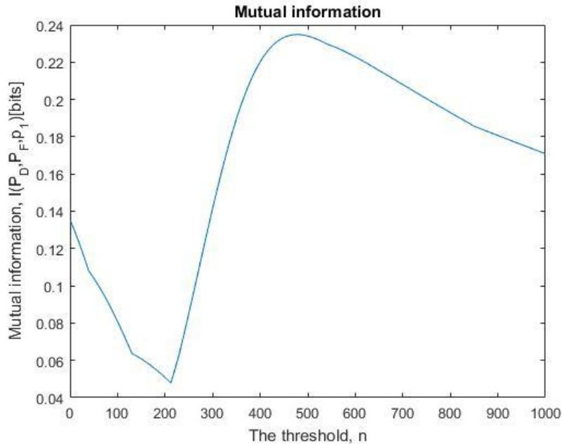
Figure 38: The mutual information in the stochastic SIMO communication system dependent on the optimal threshold,  $\eta$  with  $T_s = 200$  s
