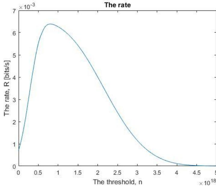
Figure 23: The rate,  $R$  with the stochastic SISO communication system when  $T_s = 150$  s
