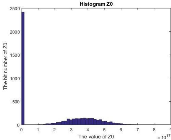
Figure 21: The distribution of  $Z_0$  in the stochastic SISO communication system when  $T_s = 150$  s
