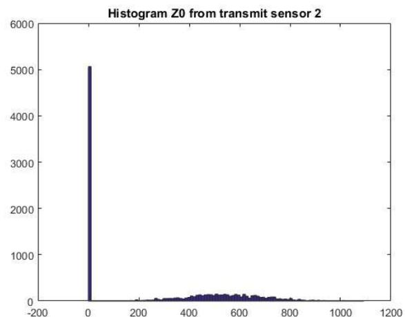
Figure 57: The distribution of  $Z_0$  from transmit sensor 2 with MIMO communication and the signaling interval,  $T_s = 300$  s
