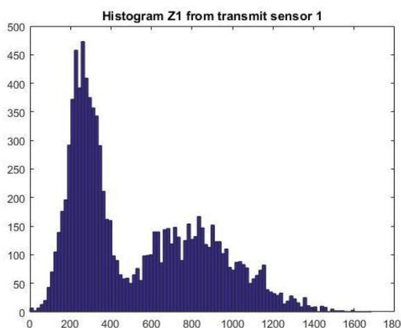
Figure 54: The distribution of  $Z_1$  from transmit sensor 1 with MIMO communication and the signaling interval,  $T_s = 300$  s
