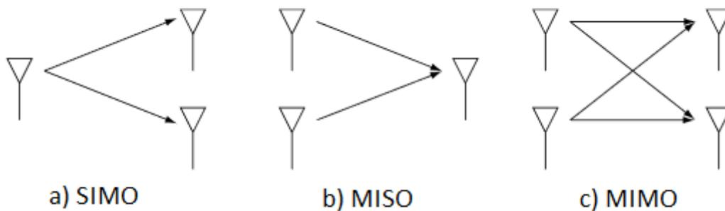
Figure 4: a) SIMO channel, b) MISO channel, c) MIMO channel
