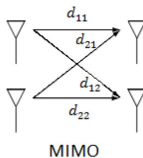
Figure 12: MIMO communication system with distances  $d_{11}$ ,  $d_{12}$ ,  $d_{21}$  and  $d_{22}$  between the transmit and receive antennas
