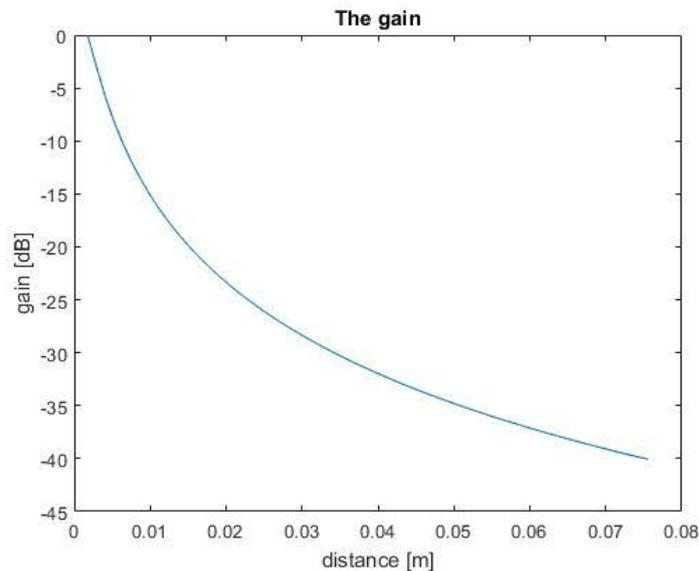
Figure 17: The gain of the concentration in the deterministic SISO communication system
