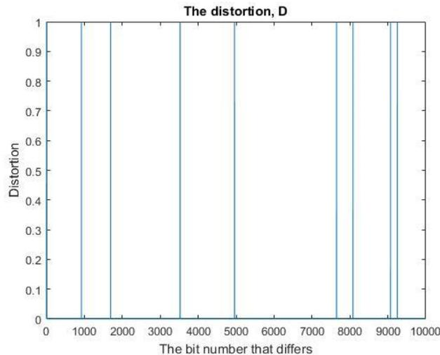
Figure 46: The distortion,  $D$  s with the stochastic SIMO communication system and signaling interval  $T_s = 250$  s
