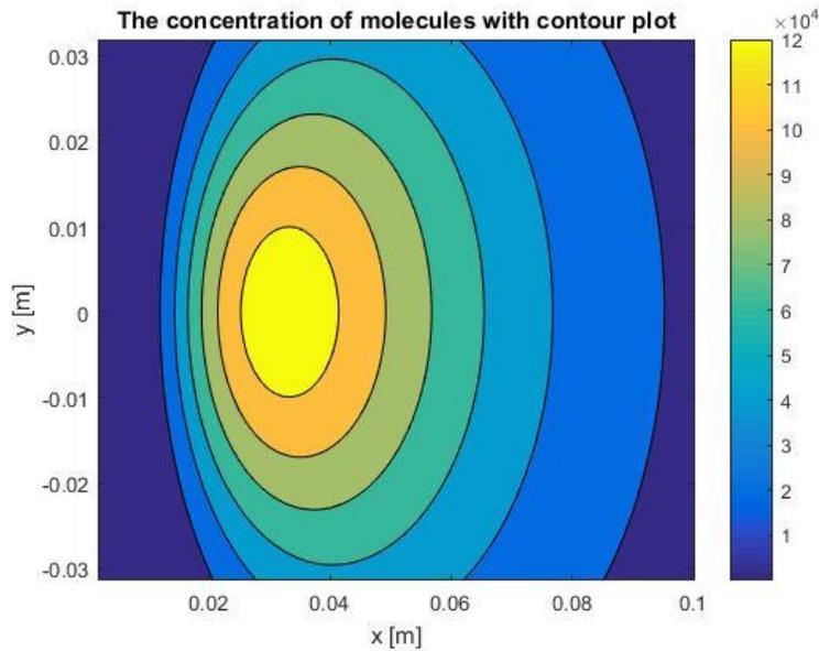
Figure 15: The concentration of the molecules in the deterministic SISO communication system dependent on the distance travelled by the molecules in the x- and y-dimension
