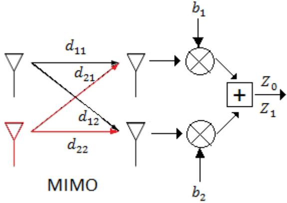
Figure 13: The MIMO system part 1 where transmitter 1 is considered
