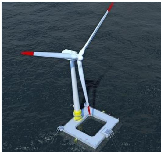
*Figure 1-3: The Damping Pool concept [5]*
