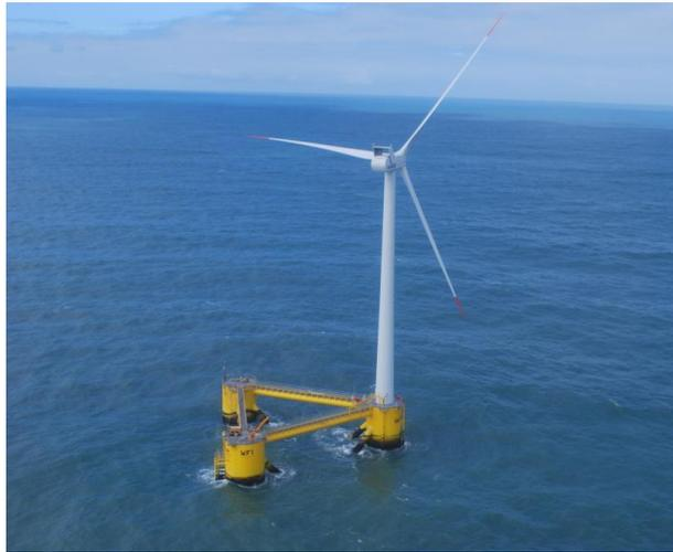
*Figure 1-2: The WindFloat concept [4]*
