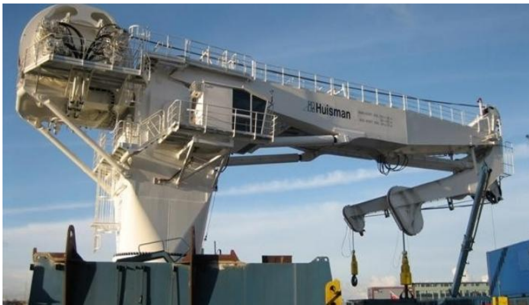
Figure 3.3: 120mt Knuckle Boom Crane( Huisman )
