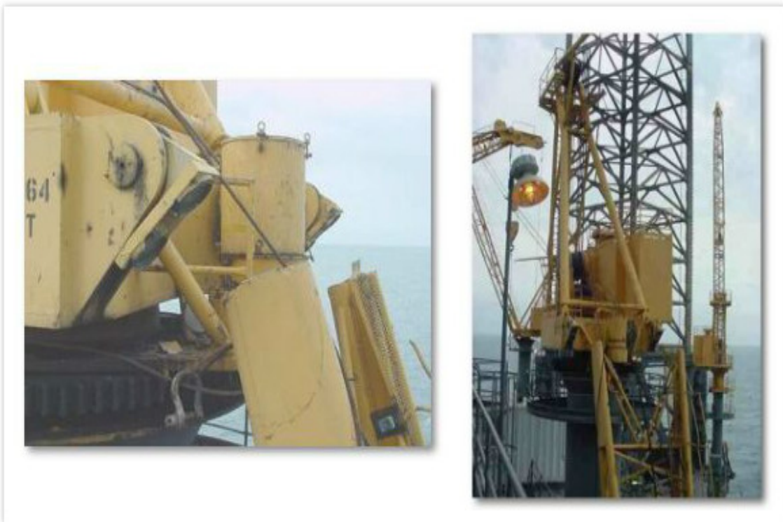
Figure 3.5: Crane Boom Failure on the jack-up rig Rowan Gorilla IV in the Gulf of Mexico( Casebook, 2008 )
