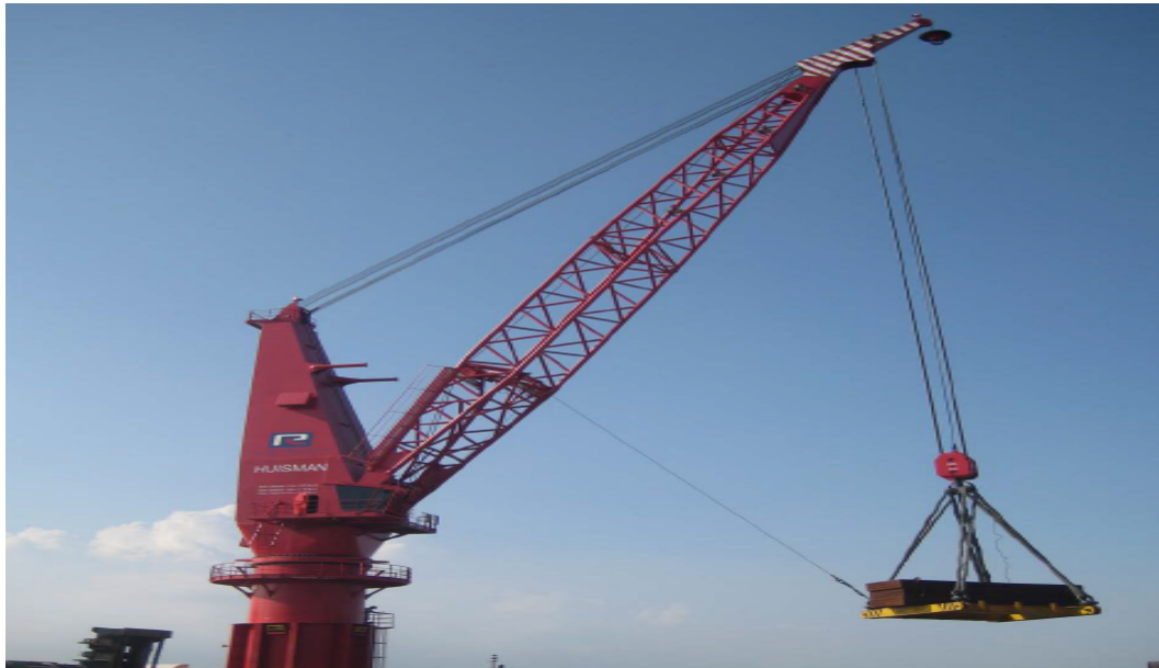
Figure 3.2: 300mt Pedestal Mounted Offshore Crane( Huisman )
