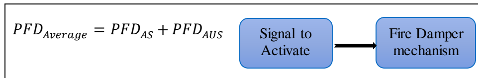
Figure 3.8: Reliability block diagram of fire damper system
