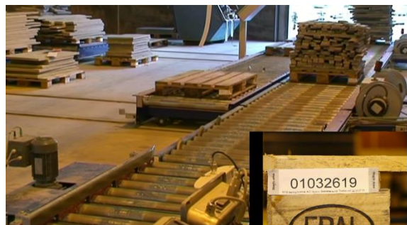
Figure 6.7 RFID tag attached to the pallet
