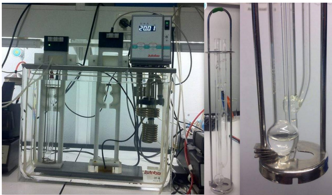
Figure 32 : Ubbelohde Viscometer Setup. On the right Alginate and \text{CaCl}_2 can be seen in viscometer bulb.
