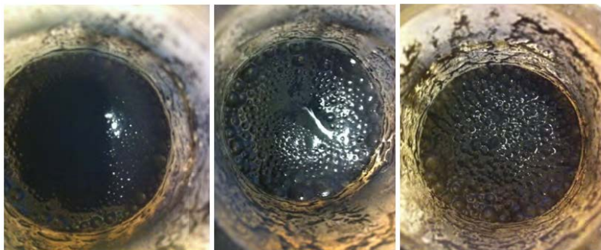
Figure 2 – Evolution of foaming in 40 mm diameter FI test container of high Carbon fly ash in figure 1 (Ollendorff 2011)
