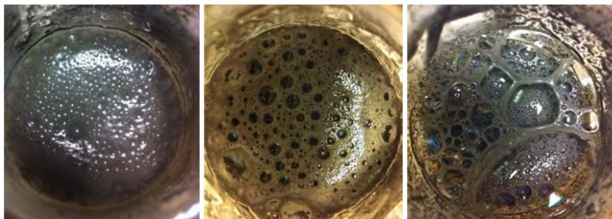
Figure 3 – Varying foam structures at stable foaming of (from left) ash No. 3, 2 and 1 in figure 1 (Ollendorff 2011)
