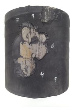
FIGURE 6.29: Coating 3 at -65°, damage
