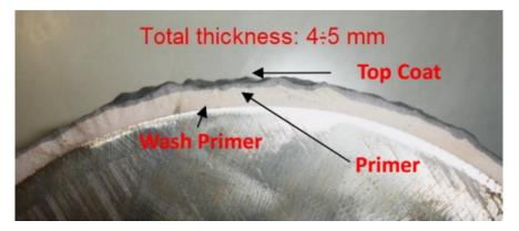
FIGURE 4.1: Cross section view of Lurask
