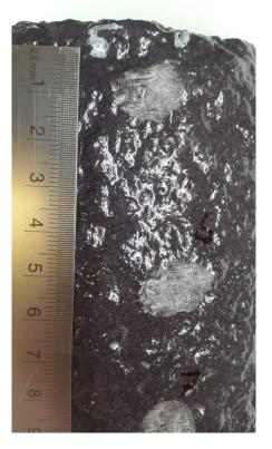
FIGURE 6.31: Coating 4 at RT, incline impact
