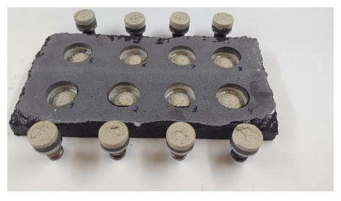
FIGURE 6.7: Coating 4 after adhesion test
