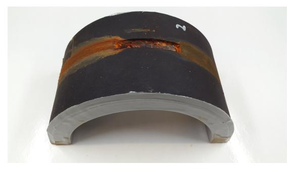
FIGURE 6.46: Coating 3 after 720 hours in the salt spray test
