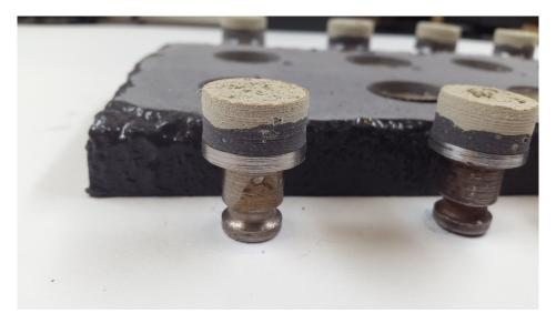
FIGURE 6.8: After adhesion test detail
