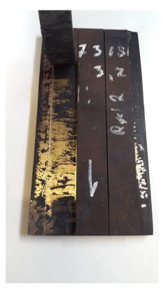
FIGURE 6.6: Coating 3 not grit-blasted
