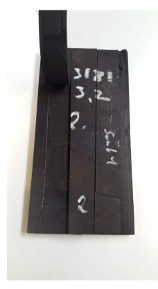
FIGURE 6.5: Coating 3 grit-blasted
