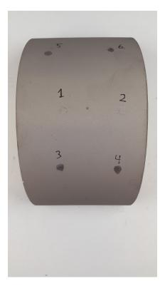
FIGURE 6.38: Coating 2 before corrosion test
