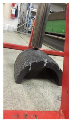
FIGURE 5.5: Impact test apparatus detail
