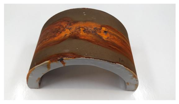
FIGURE 6.45: Coating 2 after 720 hours in the salt spray test
