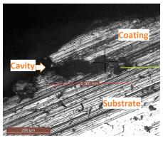
FIGURE 6.49: Coating 2, Corrosion underneath the coating
