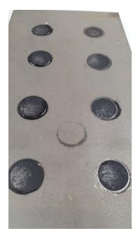
FIGURE 6.4: Fracture surface of Coating 2
