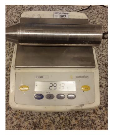
FIGURE 5.3: Indenter used for the impact test
