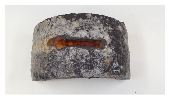
FIGURE 6.47: Coating 4 after 720 hours in the salt spray test
