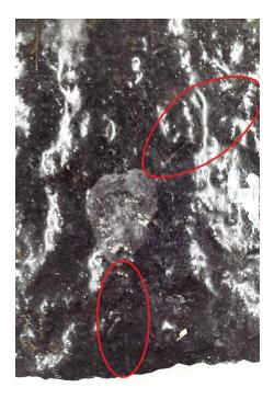
FIGURE 6.34: Coating 4 at -65°C, cracks
