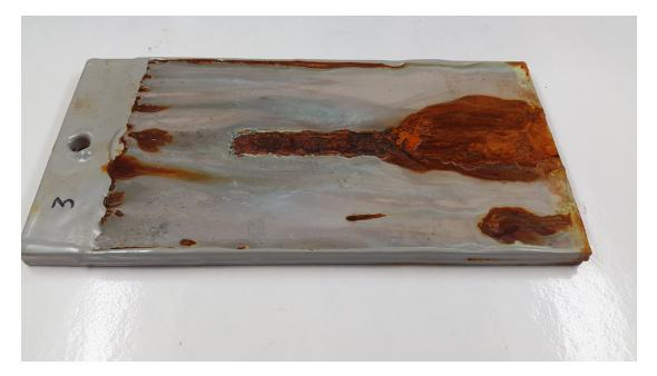
FIGURE 6.44: Coating 1 after 720 hours in the salt spray test
