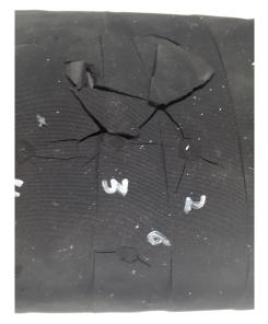
FIGURE 6.26: Coating 3 at -65°C, 7 impacts FIGURE 6.27: Coating 3 at -65°, impact 2,3,6
