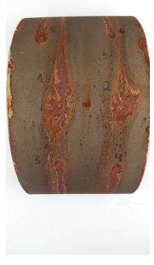
FIGURE 6.39: Coating 2 after corrosion test
