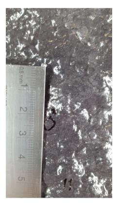
FIGURE 6.30: Coating 4 at RT, flat impact
