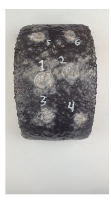
FIGURE 6.43: Coating 4 after corrosion test
