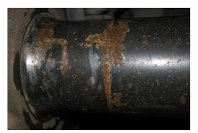
FIGURE 1.2: Corrosion on an axle
