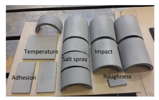
FIGURE 5.8: A selection of the samples for testing
