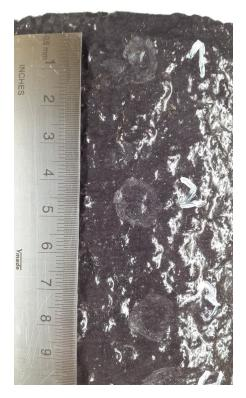
FIGURE 6.32: Coating 4 at -25°C, flat impact
