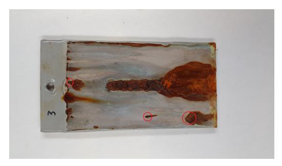
FIGURE 6.52: Coating 1 after 720 hours in the salt spray test, with highlighted defects
