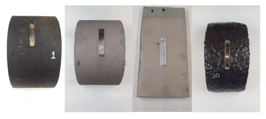
FIGURE 5.7: The aperture in all four coatings
