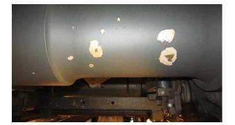
FIGURE 1.1: Impact damages on an axle
