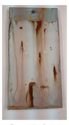
FIGURE 6.37: Coating 1 after corrosion test
