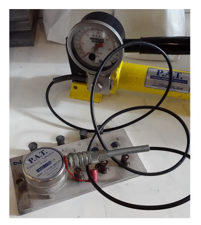
FIGURE 5.2: Pull-off test apparatus
