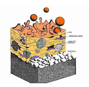
FIGURE 3.2: General Thermal Spray Coating build-up on the substrate
