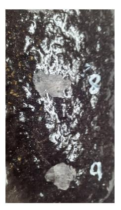
FIGURE 6.35: Coating 4 at -65°C, Cracks
