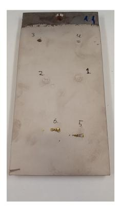
FIGURE 6.36: Coating 1 before corrosion test
