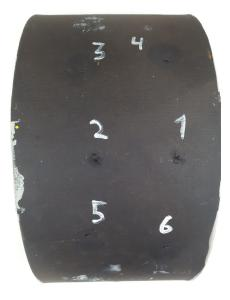
FIGURE 6.41: Coating 3 after corrosion test
