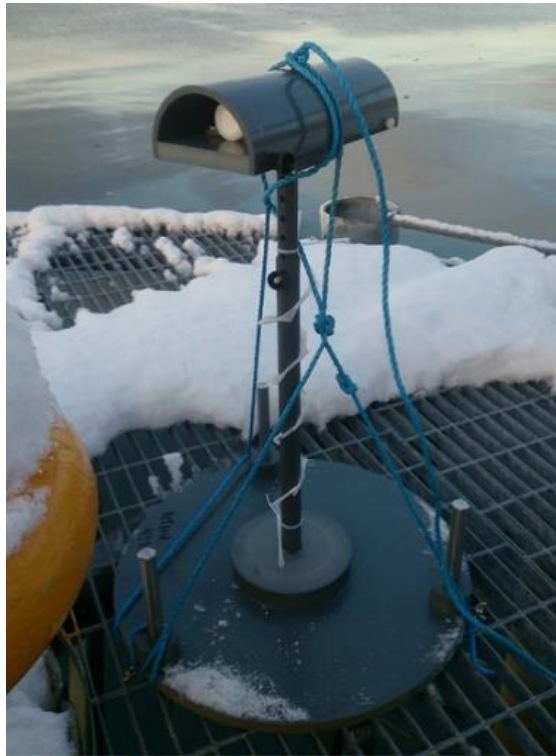
Picture 12. The equipment the DGTs were inside during sampling.
