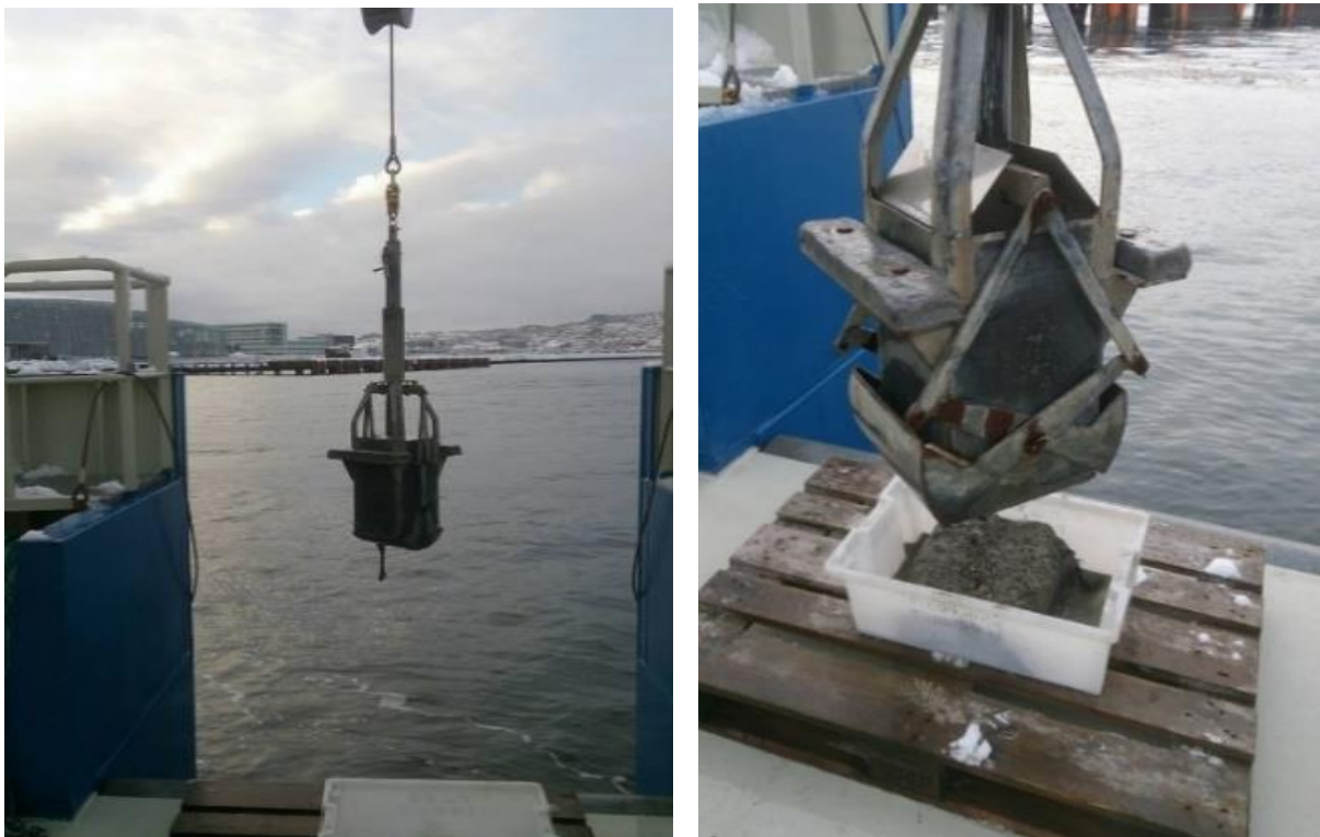
Picture 10. Sediment sampling with box corer 02.02.16. Photos by: Hilde Alida Hammer.
