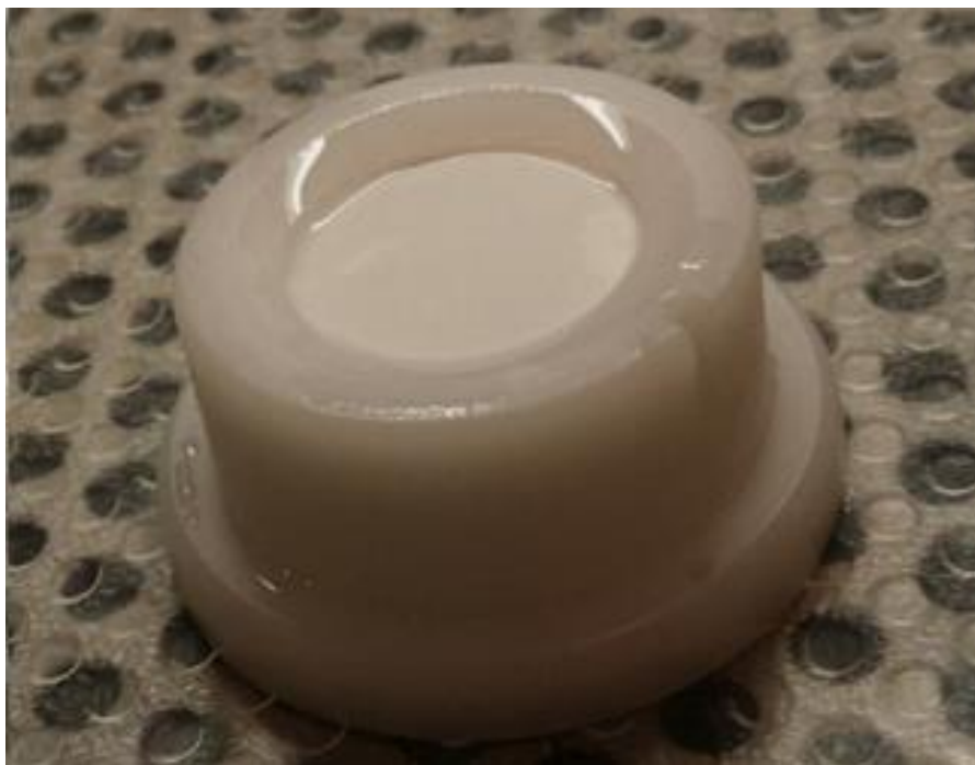
Picture 8. A completed DGT can be seen. Photo: Hilde A. Hammer.
