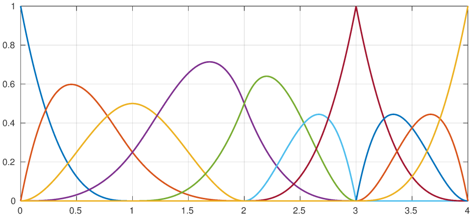
Figure 3.1: Cubic B-spline basis functions calculated from the knot vector \Xi = [0, 0, 0, 0, 1, 2, 2, 3, 3, 3, 4, 4, 4] . Some knot values are repeated, and the continuity properties of each B-spline basis function are depending on the multiplicity of each knot.
