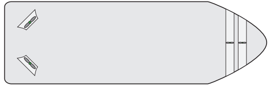
Fig. 4. Thruster layout of the simulated vessel
