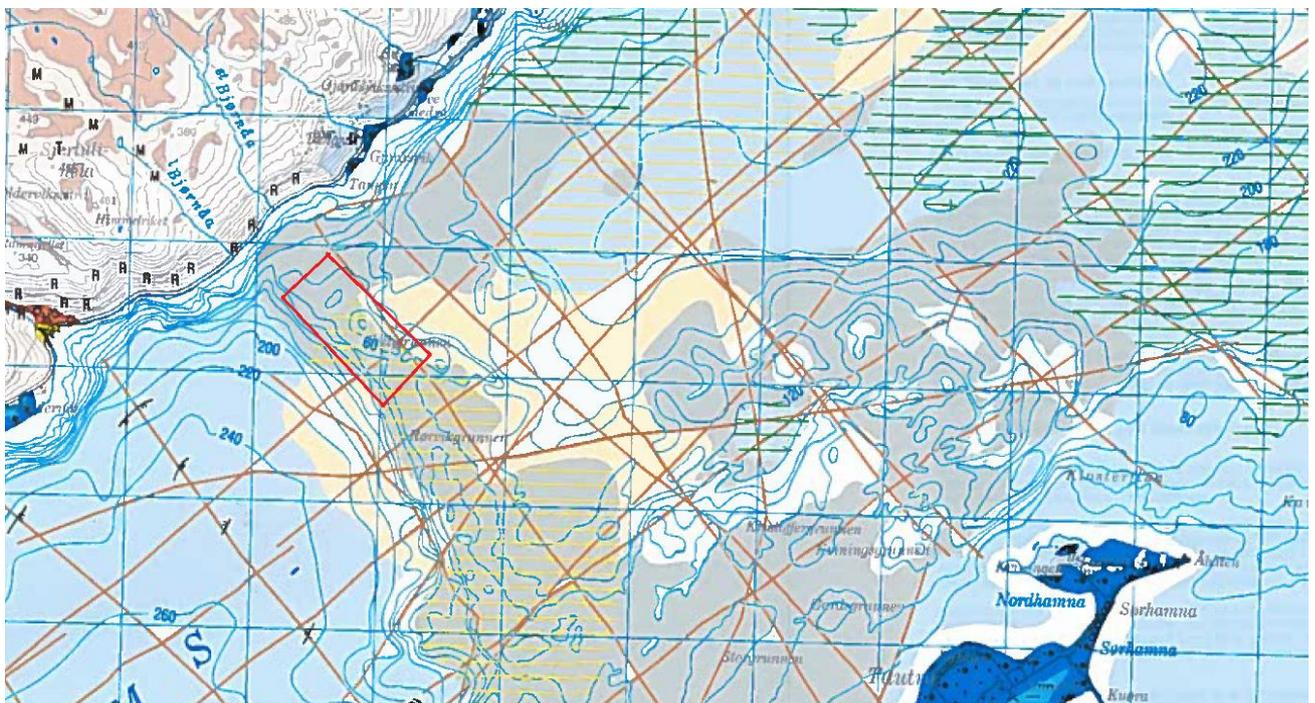
Figure 1: Geological map over the Tautra ridge provided by NGU. Scale 1:50 000. The red box indicates the area surveyed during the cruises 25th and 26th of June 2015. The colours within the box indicates a seafloor covered in till deposits in a relatively thin layer (grey/green colour) and glaciofluvial deposits (light yellow). White areas indicates bedrock. Source: (Reite and Olsen, 2002).
