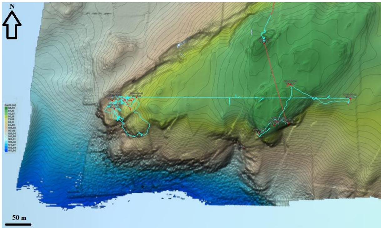
Figure 10: Digital terrain model from survey done at Høøyskjæret in Beitstadfjord 19<sup>th</sup> of May 2015. Red and blue line indicates transect of the ROV. Red colour = no video coverage, blue = video coverage. Line in lower left corner indicates 50 m distance. Dark green is approximately 35 m depth, dark blue and light blue is 200 m depth or more. Contour lines indicates 2 m interval change in depth. Upper left arrow indicates northwards direction.
