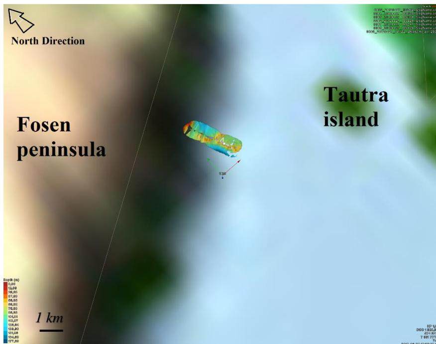
Figure 7: Area covered by MBES data from FFI cruise in 2012, processed in NaviModel 4. Black line in lower left corner of the figure indicates 1 km scale. Lower left corner indicates colour scheme for depth in the digital terrain model (DTM), where yellow-orange indicates around 65 - 70m depth. Upper left corner shows northward direction.
