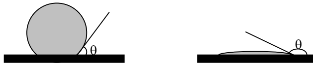
Figure 3.1 A liquid droplet in equilibrium with a horizontal surface surrounded by a gas. The wetting angle \theta between the horizontal layer and the droplet interface defines the wettability of the liquid. To the left: A non-wetting fluid with 0 < \theta < 90 . To the right: A wetting fluid with 90 < \theta < 180
