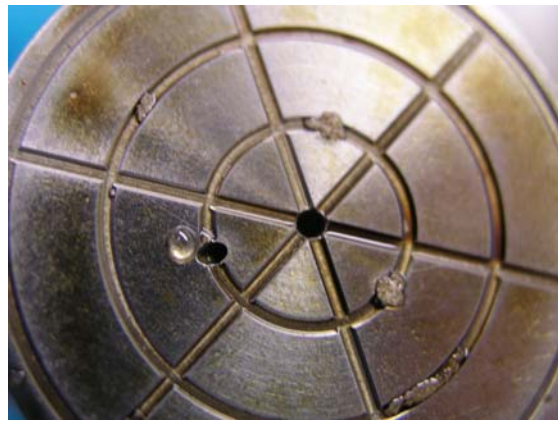
Figure 39. Pictures of the core holder inlet after microfibrill flooding. Microfibrils has blocked two of the inlet pipes.
