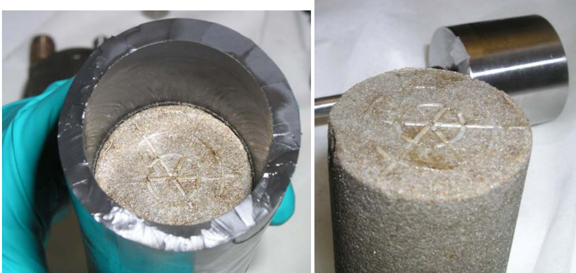
Figure 38. Pictures of the core after microfibrill flooding
