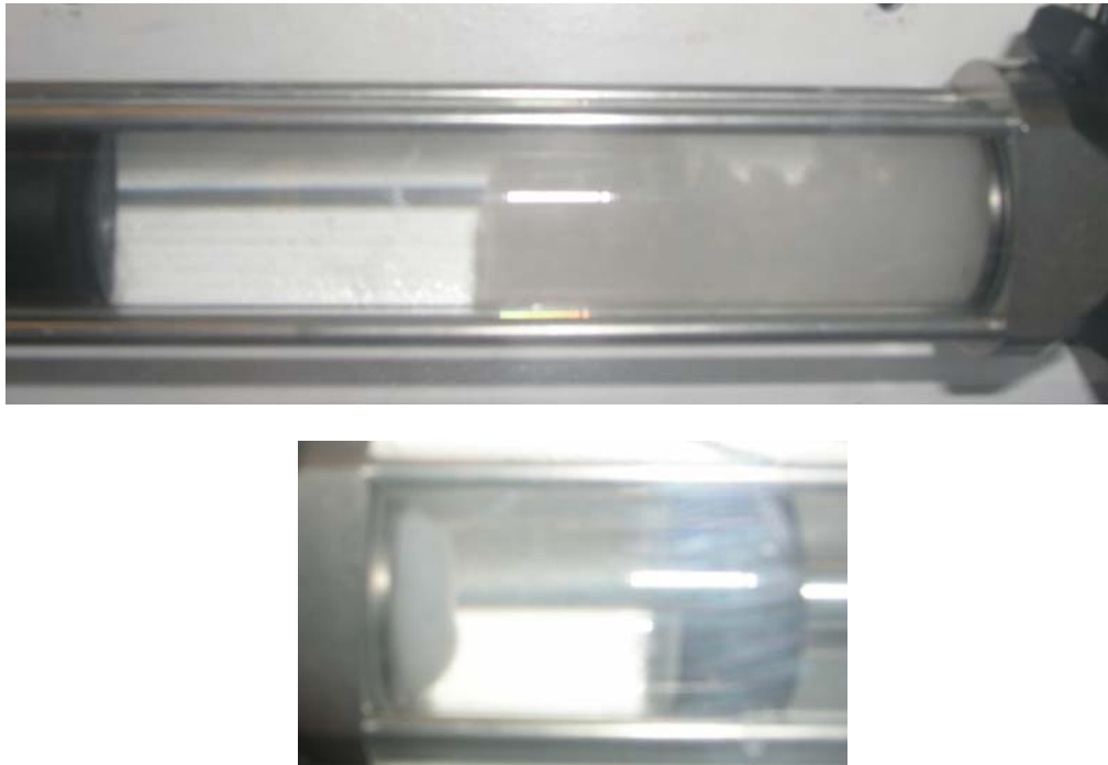
Figure 37. Pictures of the pump cylinder under microfibrill flooding. At the top the microfibrils have separated out of solution. In the bottom picture a microfibril-cake has formed blocking the outlet.
