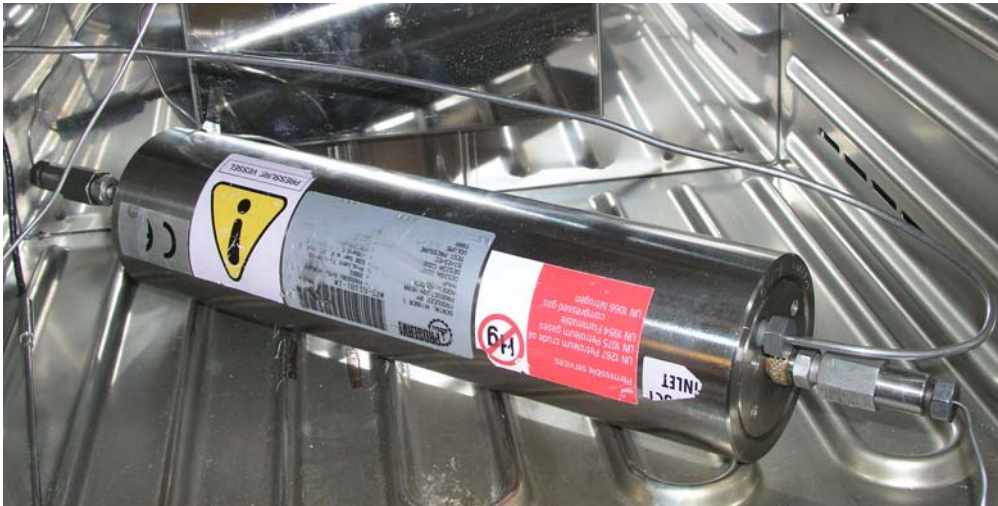
Figure 18. Picture of core holder completely mounted in heating cabinet.
