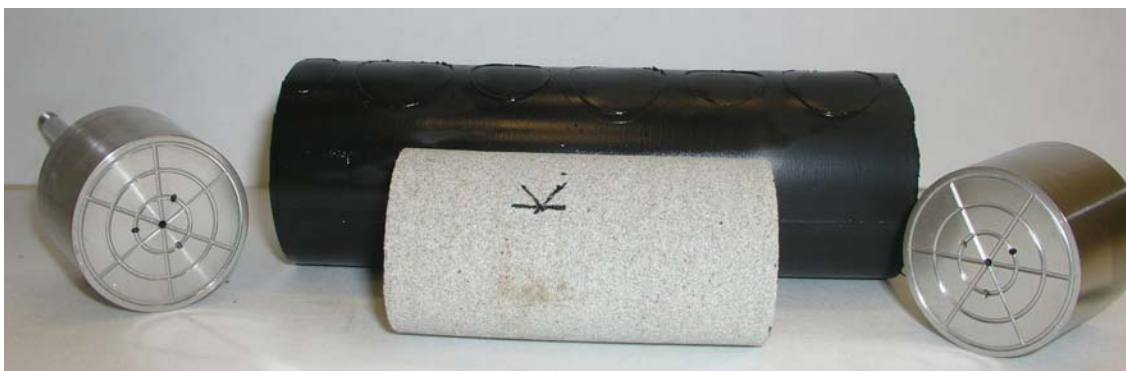
Figure 19. Picture of the sleeve, a core and the two inner end pieces.
