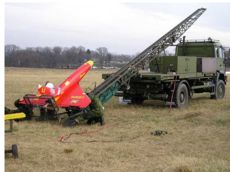
Fig. 1. A Banshee UAV ready for launch. Photo: Danish Forces Joint UAV Team
