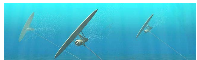
Figure 5: The kite-like turbine Deep Green [4]
