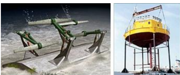
Figure 2: (a) The Pulse-Stream generator [6] (b) The Kobold turbine[13]
