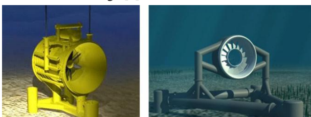
(a) Rotech Tidal Turbine [3] (b) Open Centre Turbine [11] Figure 7: Enclosed tips type turbines
