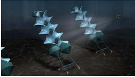
Figure 6: Flumill's Helix screws [2]
