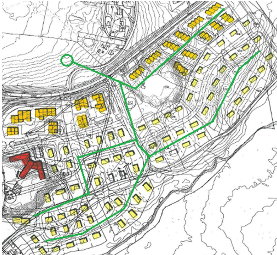
Figure 16. Sketch of circuit A in green; the circle on the top symbolizes the heat pump.
