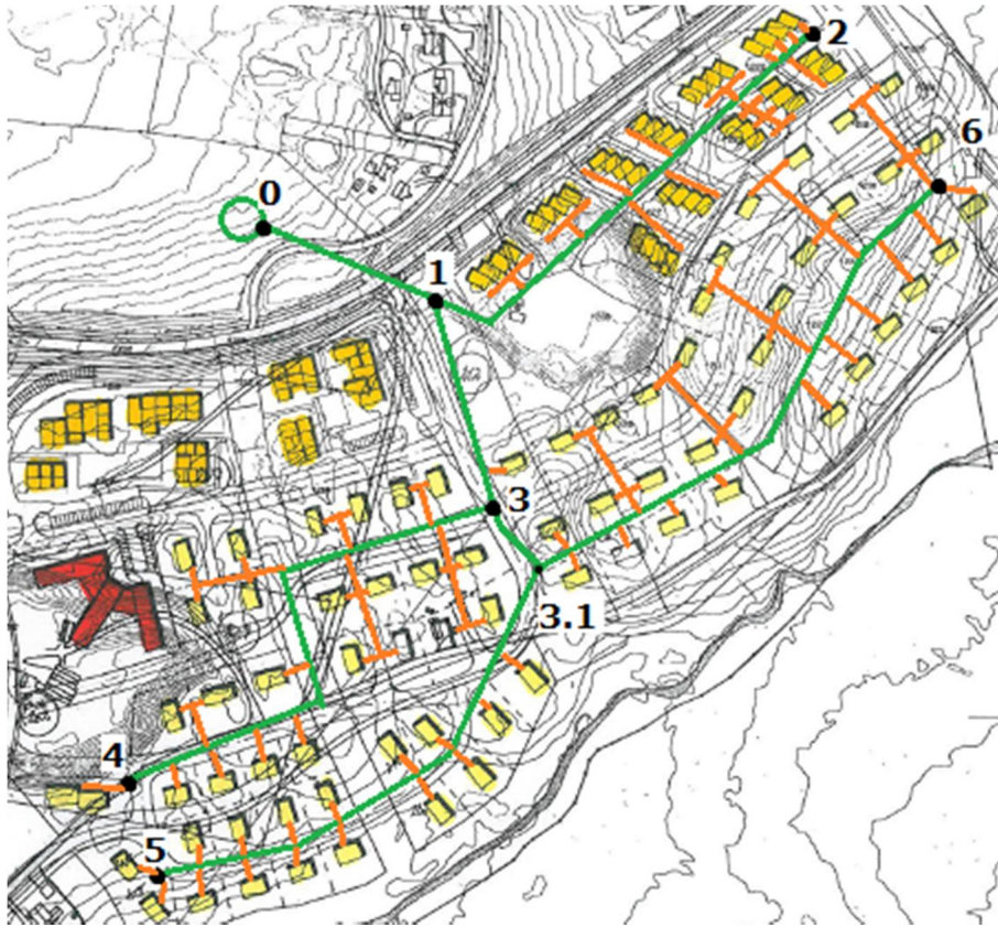
Figure 33. Sketch of circuit A with nodes. The green lines correspond to the primary circuit and the orange ones to the terminals into the houses.
