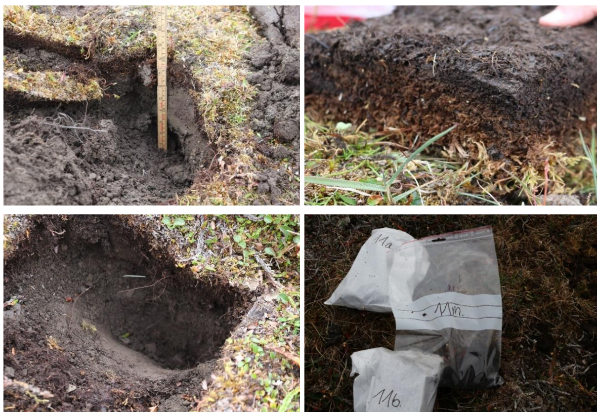
Figure 6. Pictures showing the soil sampling in Svalbard (August 2015): Soil profile (top left), surface soil sample (top right), mineral soil sample (bottom left), sample storage (bottom right).
