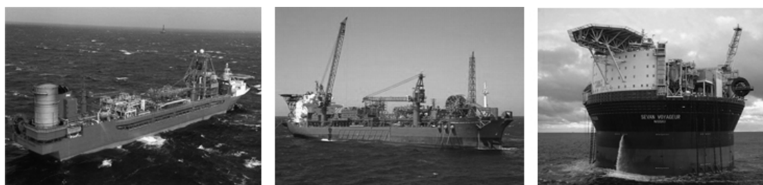
Figure 3.1: From left: Petrojarl Foinaven (conversion w/turret mooring), Petrojarl Cidade de Rio das Ostras (conversion w/spread mooring) and Voyageur Spirit (new build w/spread mooring)
