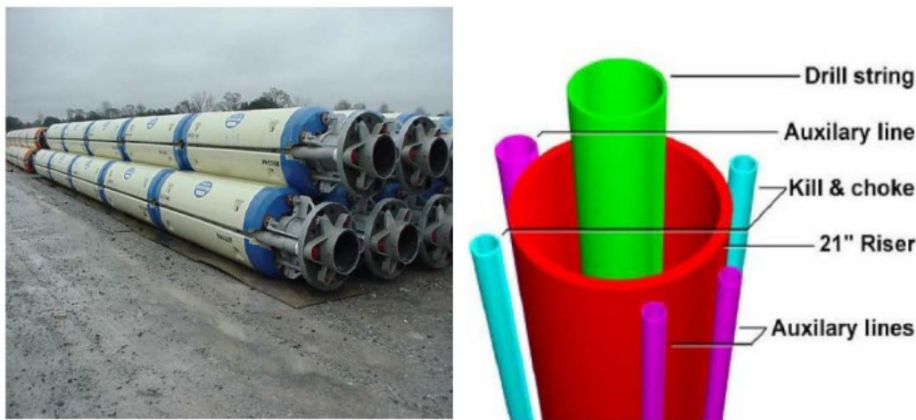
Figure 2.2: Drilling risers with buoyancy modules to the left - 3D figure of the riser, drill string and kill/choke/auxiliary lines to the right [2]
