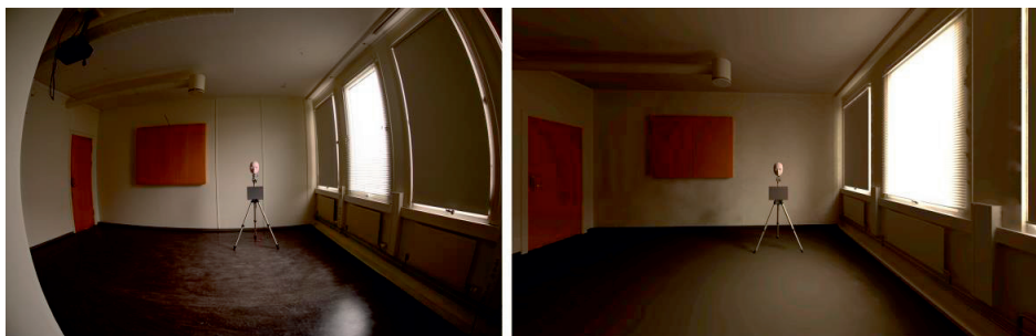
Figure 3-7. Experiment 3 with achromatic and coloured 3D objects (Venetian masks) presented in real room and simulated in Rhinoceros and DIVA programmes.
