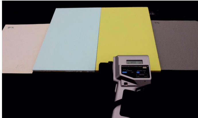
Figure 4-4. Example of the luminance measurements of two samples of the paints used in scale models.
