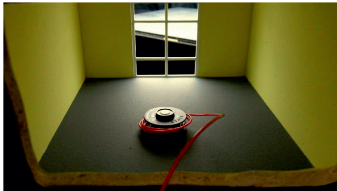
Figure 4-5. Measurement of illuminance inside the yellow scale model at floor level.
