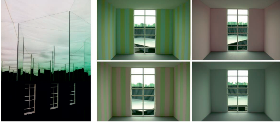
Figure 4-1. Experiment 1 with scale models inside the Artificial Sky (to the left). Example of the room interiors (one-coloured and striped).
