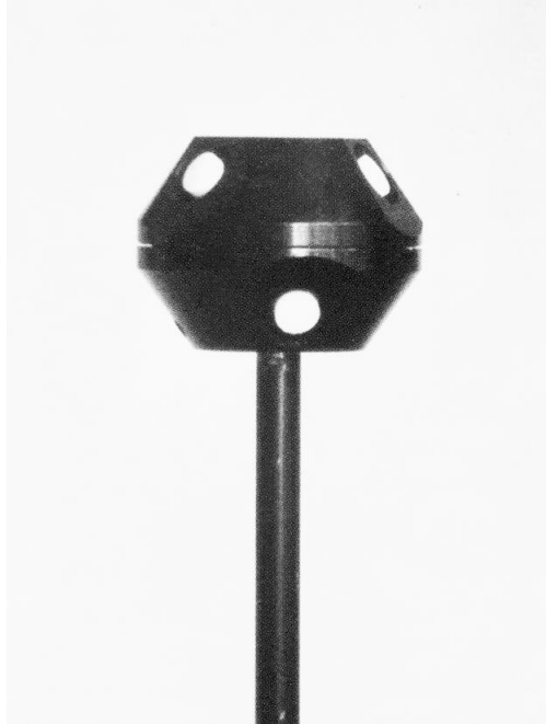
Figure 2-5. Vertical axis cubic illumination metre. Six silicon photodiodes are aligned on the faces of a cube and tilted so that one long axis is vertical. Adapted from Cuttle (2008). Adapted with permission.
