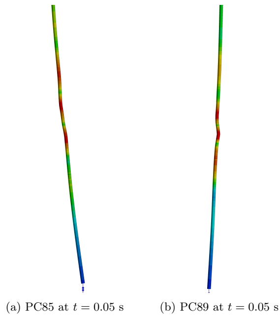
Figure C.2: Deformation of PC-riser
