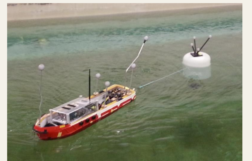
Fig. 3: CS Enterprise I and the iceberg model during a test in the MC Lab at NTNU.
