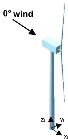
Figure 3.1: The axes orientation of the tower support at mudline (Jonkman and Buhl Jr., 2005).
