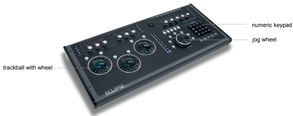
Figure 2-6: Organisation of information: Control surface Eclipse CX by JLCooper Electronics. The product is designed for precision control of colour correction and editing software. The device features abundant controls including three distinct trackballs made of Teflon (for controlling the hue in the highlights, midtones, and shadows), a numeric keypad for quick timecode entry, different types of buttons and keys, dials, and a jog wheel with a concentric shuttle ring (allowing the user to shuttle through audio and video media). The wheel around each trackball lets the user adjust the luminance. Information and illustration are available on: https://jlcooper.com/_php/product.php?prod=eclipsecxm (accessed 18 September 2014).
