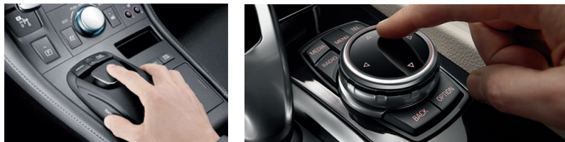
Figure 3-8a (left): Haptic perception in a driving context: Remote touch haptic controller in Toyota’s Lexus cars. The controller is similar to a computer mouse or joystick and enables one-handed operation while allowing the driver to concentrate on the road. Figure 3-8b (right): The BMW iDrive touch controller is designed as a control wheel and enables users to easily display and control in-car information while keeping attention on the road.
