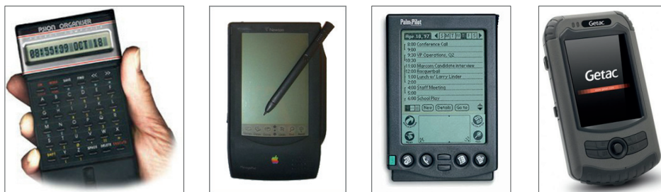
Figure 3-18: From left to right: Psion 1, 1984. The device allowed users to store contact information and a schedule and included a clock and calculator. Newton MessagePad100, 1993. Apple introduced the device. It was the first PDA with handwriting recognition. Palm Pilot, 1996. The device was economically more successful than Apple's product. Getac PS535F, 2009. The handheld device is a compact rugged PDA for industrial use that is based on the Windows Mobile platform.
