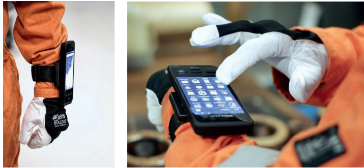
Figure 7-5: The explosion-proof smartphone Impact X can be mounted on a wrist cradle and enables hands-free working. (Photo: Bartec Pixavi)
