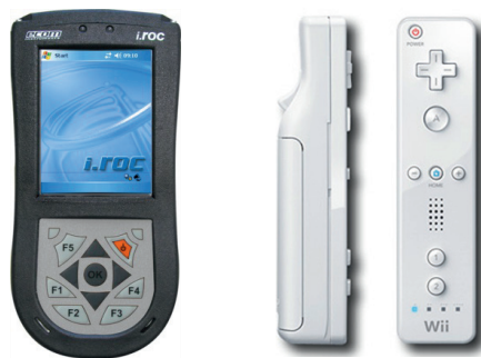
Figure 3-1a (left): Industrial PDA i.rock 420 Ex with an embossed keyboard that gives tactile feedback. The navigation buttons have an arrow-shaped form and indicate the direction of movement. Figure 3-1b (right): Nintendo Wii remote controller with its typical cross-shaped directional pad.
