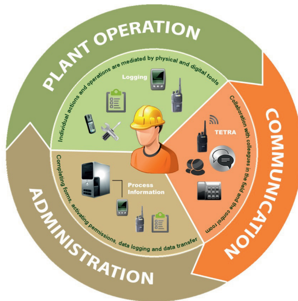
Figure 6-6: Plant operating, communication, and administration (actions) are performed as part of the overall activity — in this case, onshore gas production. Each action includes concrete operations enhanced by the use of physical artefacts, such as paper and pen, and by IT, such as stationary equipment, a handheld PDA, and a TETRA terminal.
