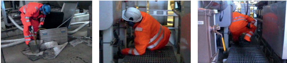
Figure 3-13: Critical body postures: Field operators often perform actions that require different body postures. The photographs show the removal of CO 2 -residues (to the left) and the controlling of valves (in the middle, to the right). In both cases, the involved operators are forced to take uncomfortable postures (Photographs: author).
