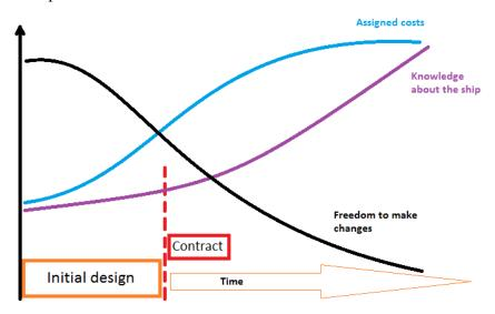
Figure 4. The visual representation of the increase in knowledge and costs while the freedom to make changes decreases, over time. As per [2][10].
