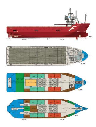
Figure 6. GA drawing of a supply vessel, taken from [24].
