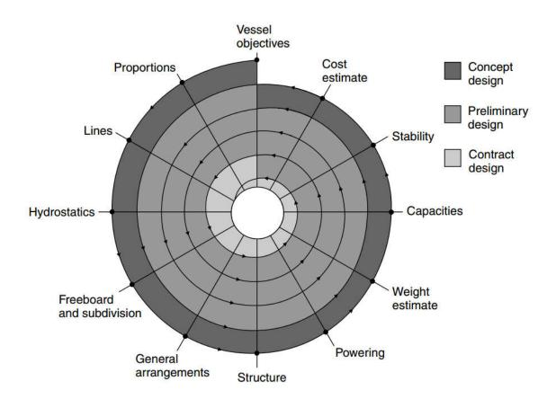
Figure 3. Design spiral, as proposed by Harvey-Evans, taken from "Ship construction" [5].
