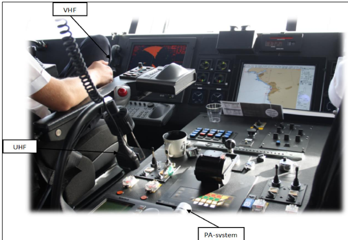
Figur 2-12 The location of communication equipment on bridge (Åfeldt Jimmy).
