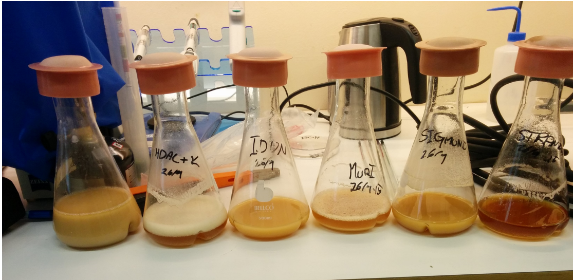
Figure 12: Kveik cultures and Idun being grown in 500 mL incubation flasks. A vial of WLP001 was suspended in 5 % ME medium before transferred to fermentation vessel. Shown from left to right are WLP001, original Hornindal, Idun, Muri, Sigmund and Stranda, 5 % ME medium for beer Experiment 1.
