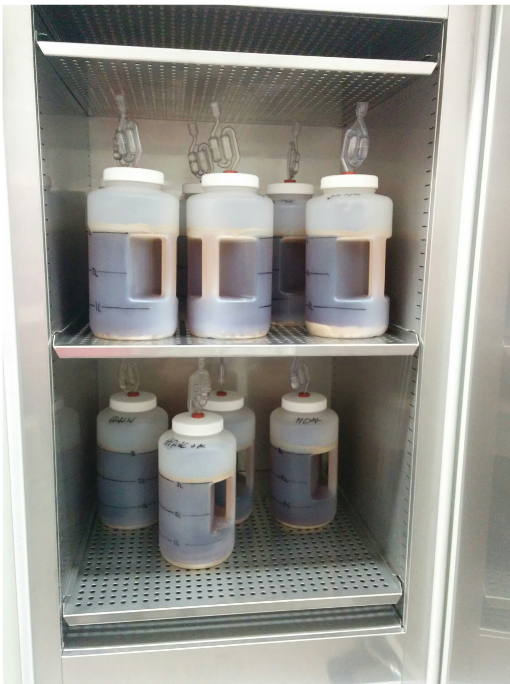
Figure 19: Incubation of experiment 2 with Kveik, Idun and WLP001 at 19 °C.
