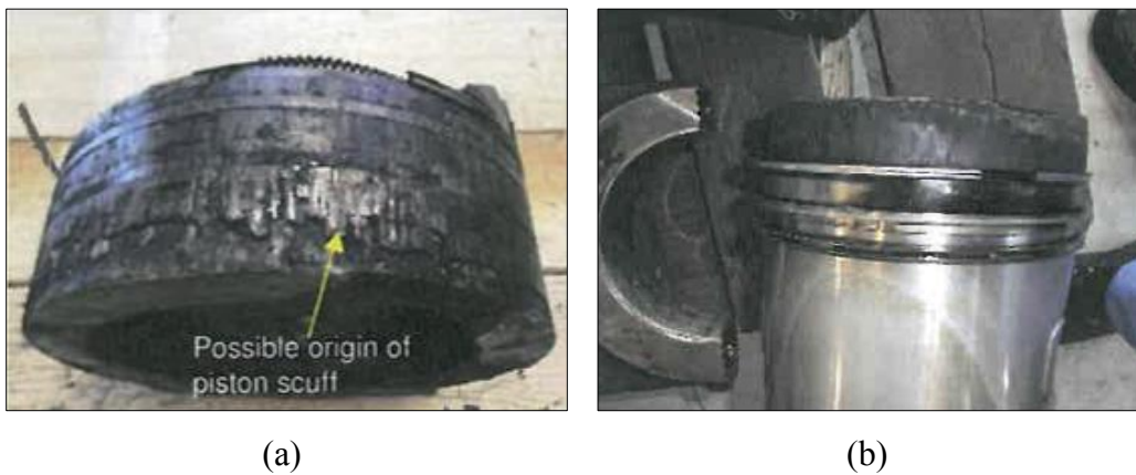
Figure 3-1: Piston scuffing and carbon deposits. Picture (a) shows piston scuffing on piston #5. Picture (b) shows deposits of hard carbon on the top land of piston #4. Courtesy of [25]
