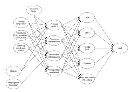
Figure 3.7: ORIM causal network model for leak freqency. Source: Øien (2001a)
