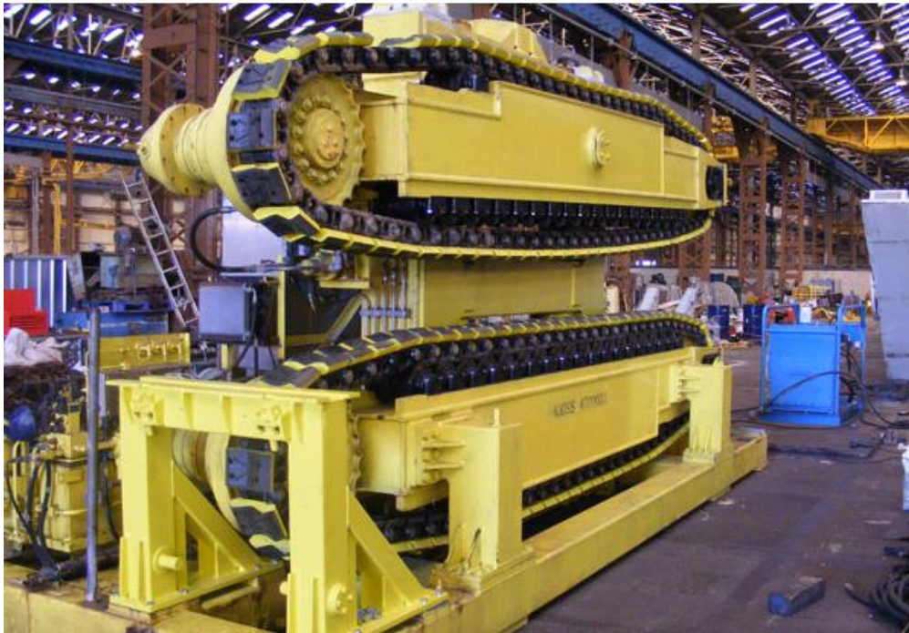
Figure 29: Tracked Cable Engine (System 2013)
