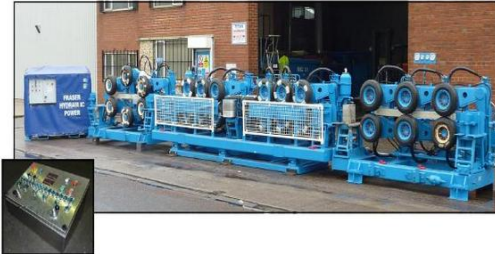
Figure 28: 12-18 Pair Linear Cable Engine (Ltd 2007)
