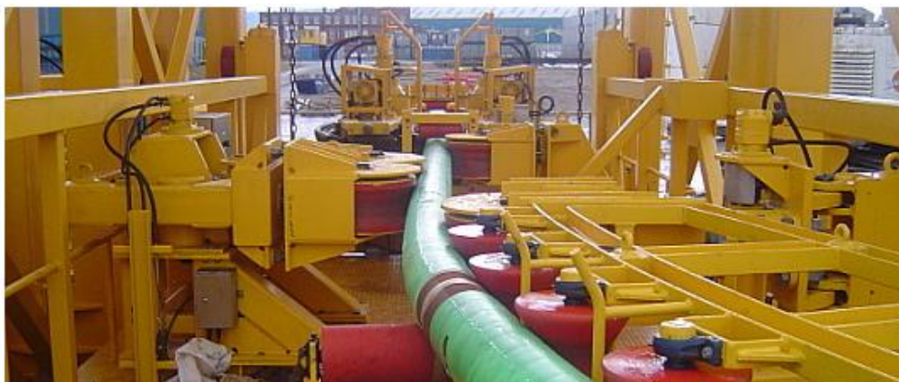
Figure 36: Roller guidance system example (System 2013)
