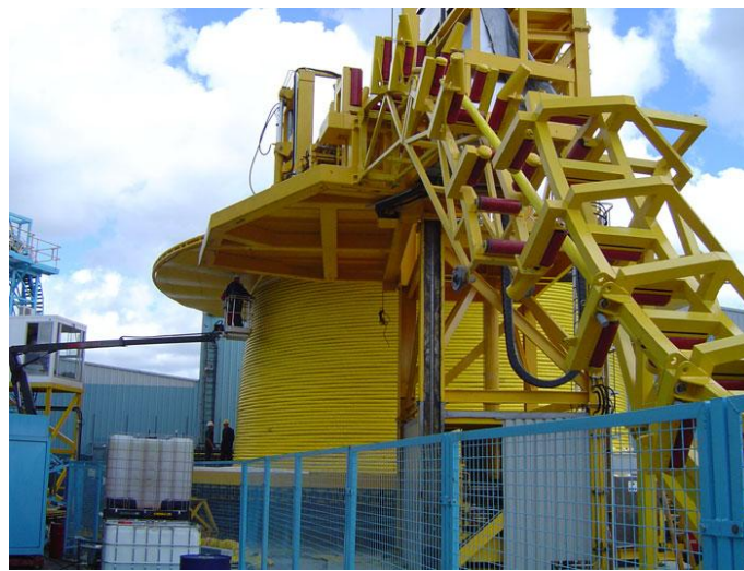
Figure 37: Cable laying machinery – guider arm (Systems 2013)
