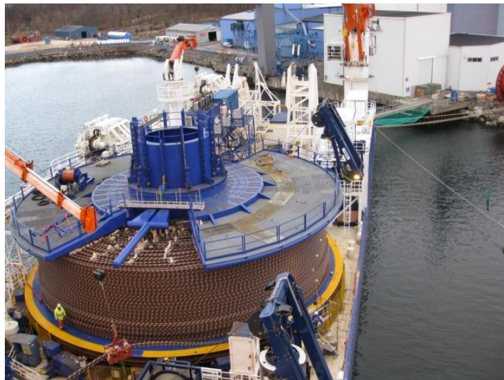
Figure 8: Horizontal cable drum spool storage system (SHIPPING 2013)
